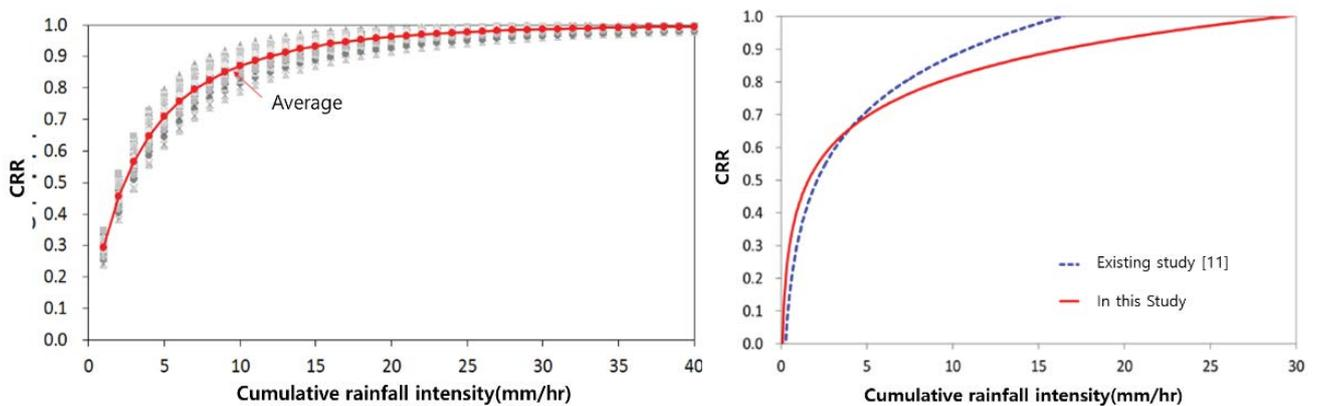
Fig. 6. Correlation between the cumulative rainfall intensity and CRR using the hourly rainfall data for the last 30 y.
