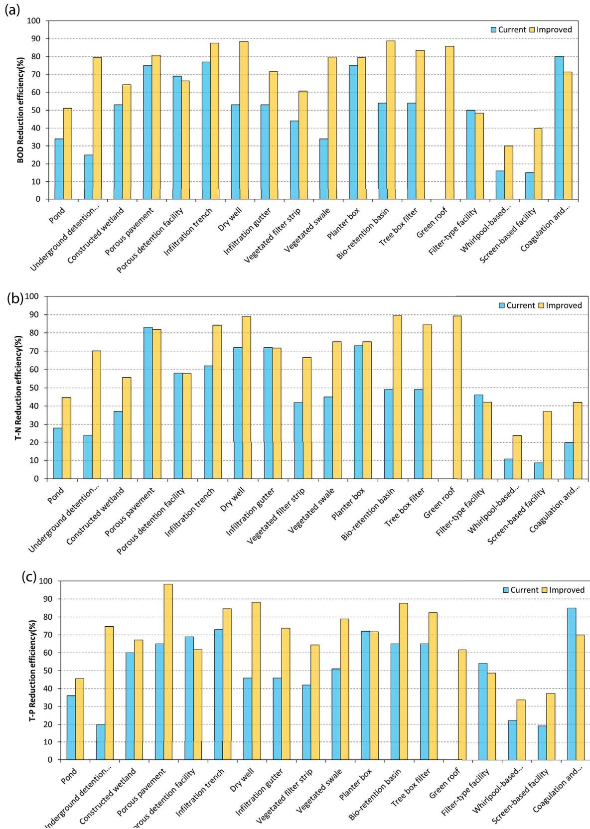
Fig. 9. Comparison between the present study and the TMDL guideline for the estimation method for the average pollutant load reduction efficiency: (a) BOD, (b) TN, and (c) TP.
