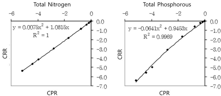
Fig. 2. Relation between the CRR and CPR of TN and TP in a constructed wetland [11].
