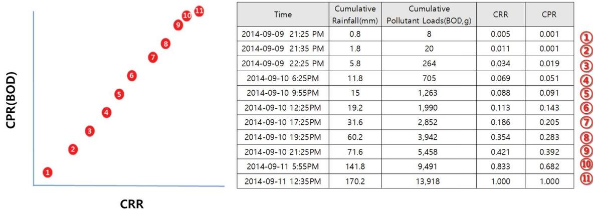
Fig. 4. Example of the determination of the regression equation for the CPR.
