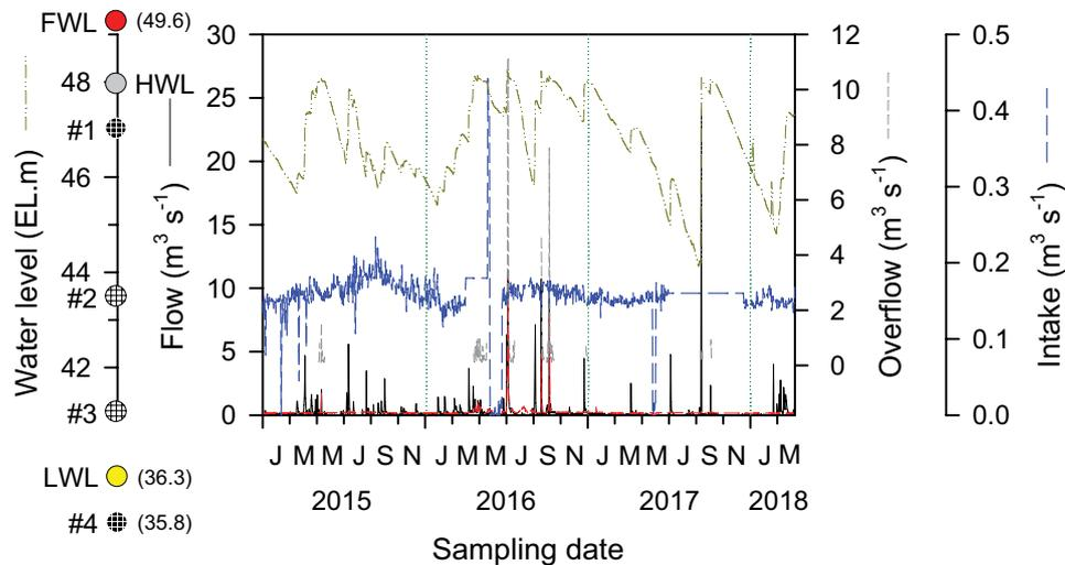
Fig. 4. Daily variation in the major hydrological factors of inflow, overflow (spillway discharge), intake, and water level in the Yeoncho Reservoir from January 2015 to April 2018. FWL: flood water level; HWL: high water level; LWL: low water level. #1–4 (EL. m): intake gate numbers in the selective withdrawal facility.
