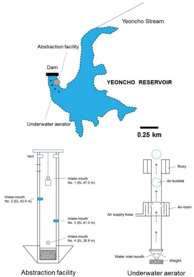
Fig. 2. Map showing the locations of the abstraction facility and the underwater aerators operating within the reservoir, and schematic diagrams explaining their detailed structures.
