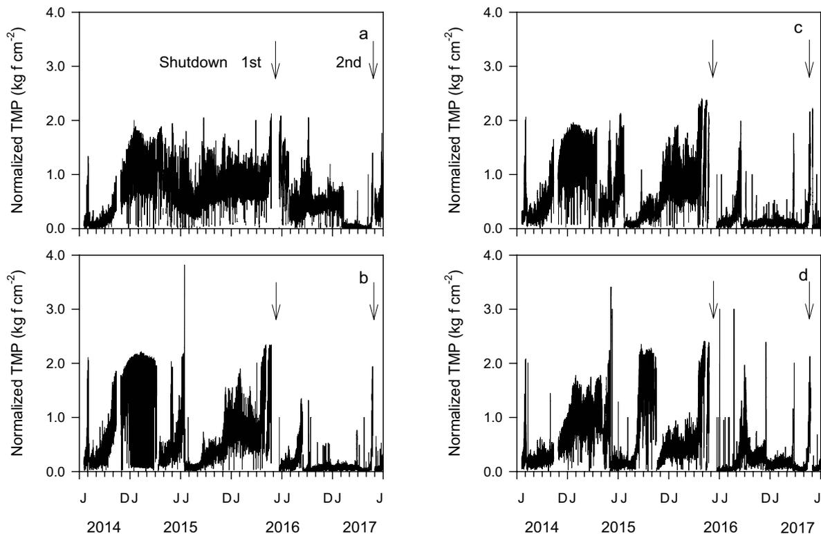
Fig. 3. Real-time fluctuations in the normalized transmembrane pressure (TMP) measured at 1 h intervals in the Yeoncho water treatment plant from July 2014 to June 2017. (a–d) represents the four membrane module lines.
