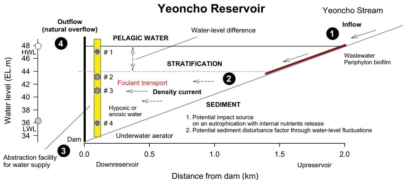
Fig. 8. Schematic diagram explaining the relationship between foulant transport from the Yeoncho Reservoir to the Yeoncho water treatment plant and the abstraction facility and underwater aerators. HWL: high water level; LWL: low water level. #1–4: intake gate numbers of the selective withdrawal facility.
