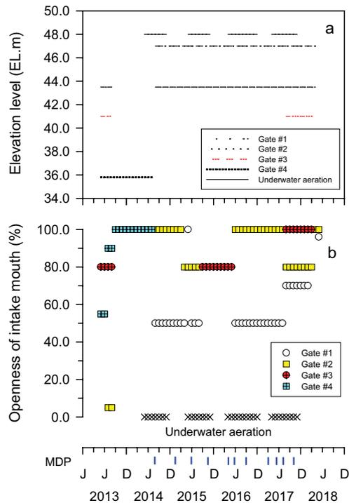
Fig. 6. Qualitative (a) and quantitative (b) results of the operation of the selective withdrawal facility and underwater aeration systems in the Yeoncho Reservoir from January 2013 to December 2018. Membrane differential pressure (MDP) refers to the time when the transmembrane pressure was severe.
