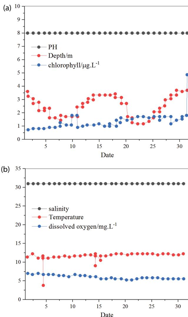
Fig. 5. Real time collection of ecological parameters: (a) depth, pH, and chlorophyll curve and (b) curve of temperature, salinity, and dissolved oxygen.
