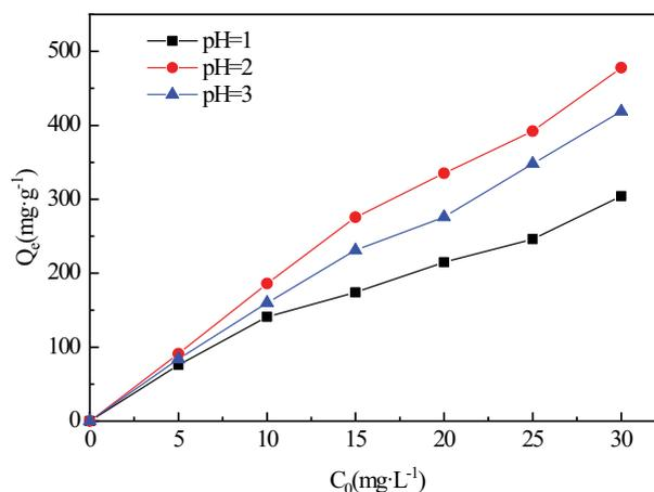
Fig. 7. Adsorption capacity in different pH T = 298 K; adsorbent dosage, 0.01 g; initial concentration, 5, 10, 15, 20, 25 and 30 mg L<sup>-1</sup>.
