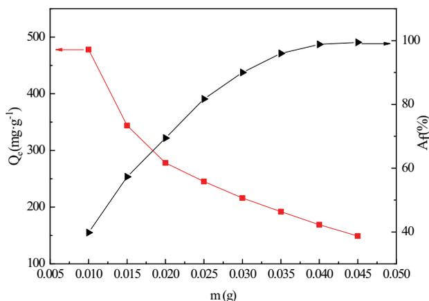
Fig. 10. Influence of adsorbent dosage on the adsorption efficiency pH = 2;  $T = 298 \text{ K}$ ; initial concentration,  $30 \text{ mg L}^{-1}$ .
