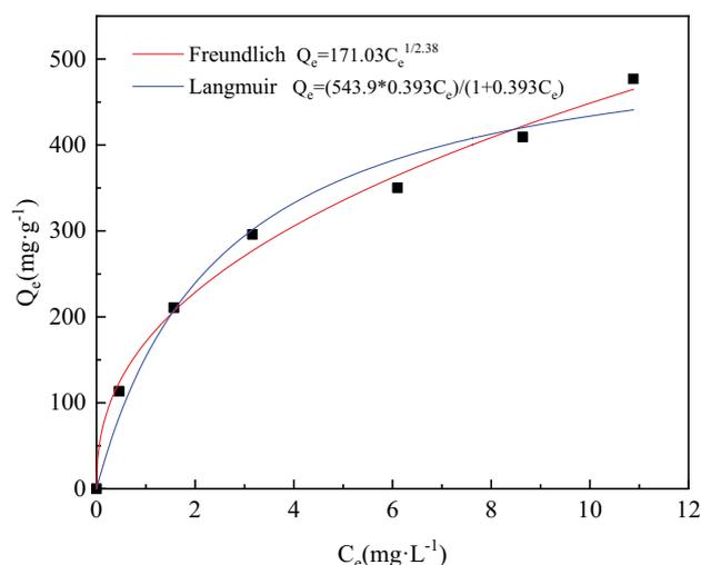
Fig. 6. Adsorption isotherm pH = 2; T = 298 K; adsorbent dosage, 0.01 g; initial concentration, 5, 10, 15, 20, 25 and 30 mg L<sup>-1</sup>.
