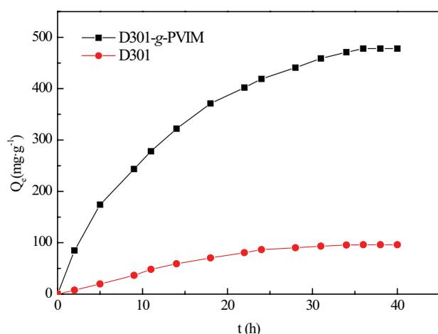
Fig. 4. Adsorption kinetics of Au(III) curves pH = 2;  $T = 298$  K; adsorbent dosage, 0.01 g; initial concentration, 30 mg L<sup>-1</sup>.
