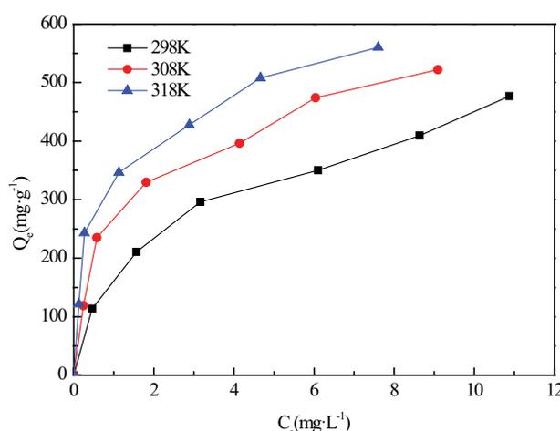
Fig. 8. Isotherms in different temperature pH = 2; adsorbent dosage, 0.01 g; initial concentration, 5, 10, 15, 20, 25 and 30 mg L<sup>-1</sup>.
