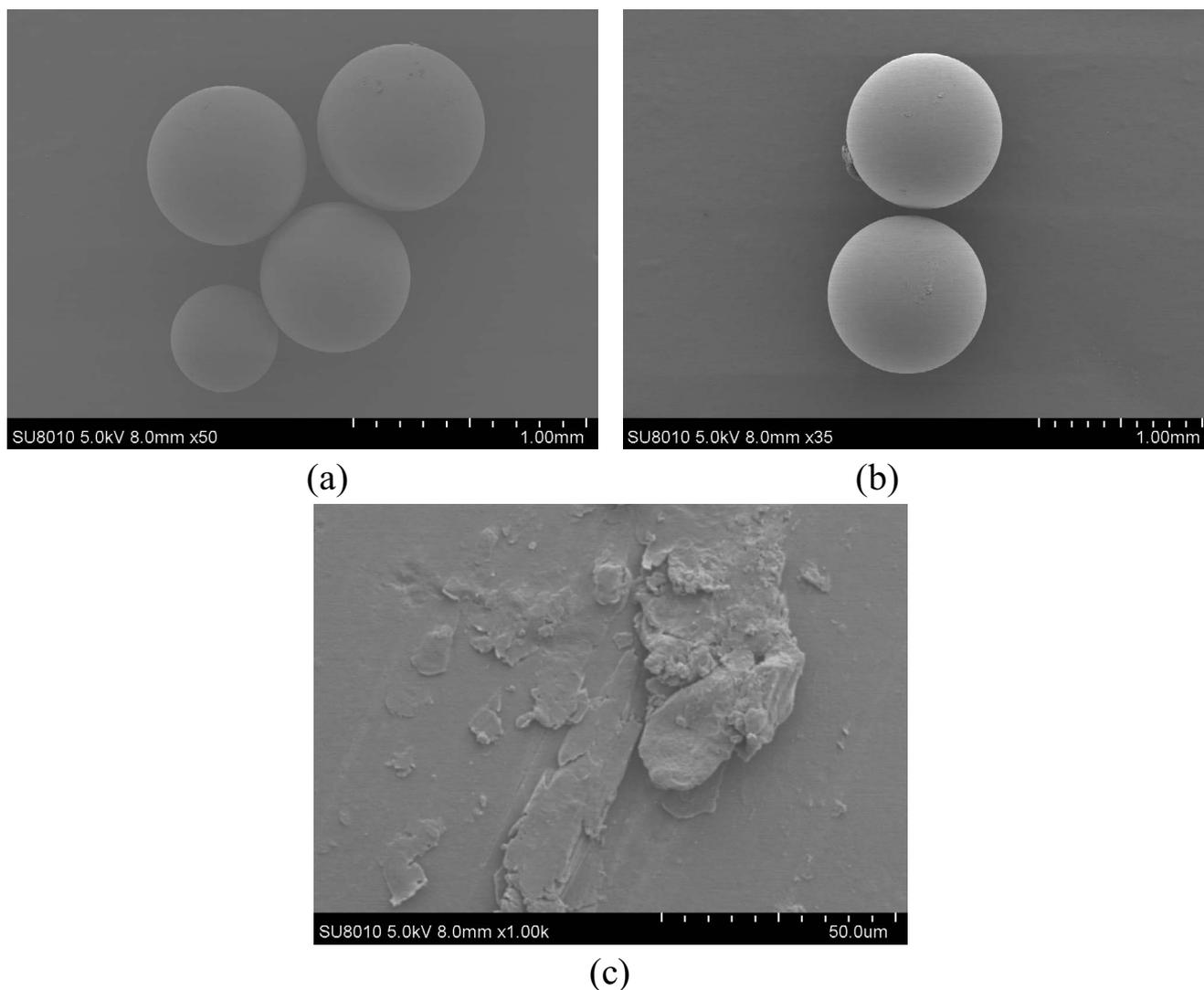
Fig. 3. SEM images of D301 (a) and D301-g-PVIM (b and c).
