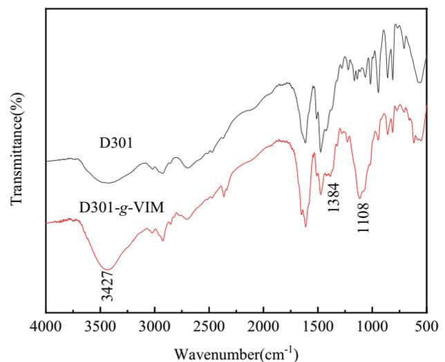
Fig. 2. FTIR spectra of D301 and D301-g-PVIM.
