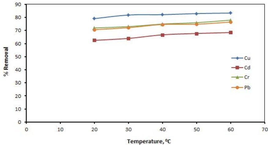
Fig. 8. Effect of temperature on the percentage removal of metal ions using potato peels. Experiment conditions: initial concentration, 100 mg/L; temperature, 20°C–60°C; adsorbent dose, 1 g; particle size, 250  $\mu\text{m}$ ; shaking rate, 150 rpm, and pH, for Cd(II) pH = 6, for Cu(II), Pb(II) and Cr(III) pH = 4.
