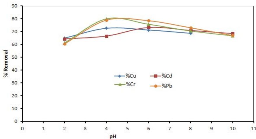
Fig. 5. Effect of pH on the percentage removal of metal ions using potato peels. Experiment conditions: initial concentration, 100 mg/L; temperature, room temperature (25°C); adsorbent dose, 1 g; particle size, 250  $\mu\text{m}$ ; shaking rate, 150 rpm; and pH 2–10.
