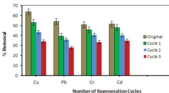
Fig. 9. Recycling study of Cd(II), Pb(II), Cu(II) and Cr(III) onto potato peels.
