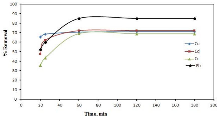
Fig. 4. Effect of time on the percentage removal of metal ions on potato peels for different metal ions solution concentrations. Experiment conditions: initial concentration, 100 mg/L; temperature, room temperature (25°C); adsorbent dose, 1 g; particle size, 250  $\mu\text{m}$ ; shaking rate, 150 rpm, and pH, for Cd(II) pH = 6, for Cu(II), Pb(II) and Cr(III) pH = 4.
