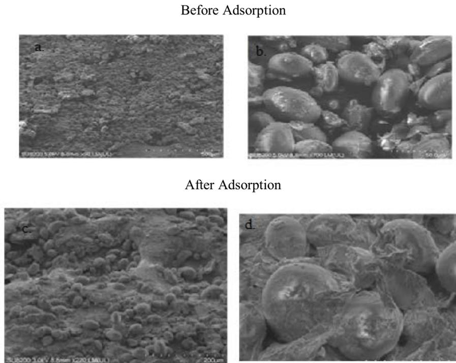
Fig. 2. SEM analysis of potato peels before and after metal ions adsorption.
