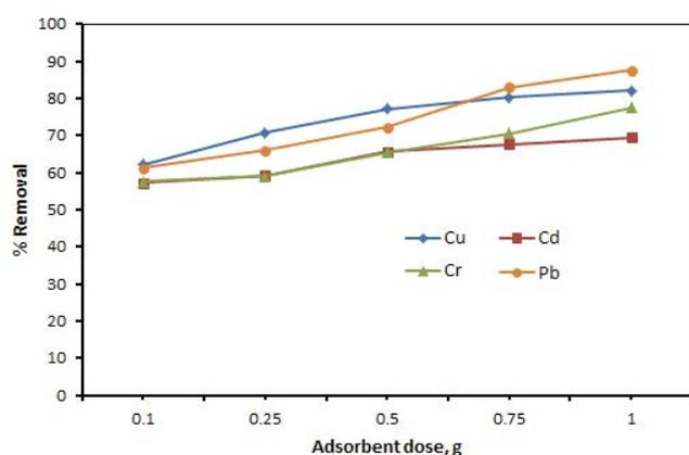
Fig. 6. Effect of adsorbent dose on the percentage removal of metal ions using potato peels. Experiment conditions: initial concentration, 100 mg/L; temperature, room temperature (25°C); adsorbent dose, 0.1–1 g; particle size, 250  $\mu$ m; shaking rate, 150 rpm, and pH, for Cd(II) pH = 6, for Cu(II), Pb(II) and Cr(III) pH = 4.
