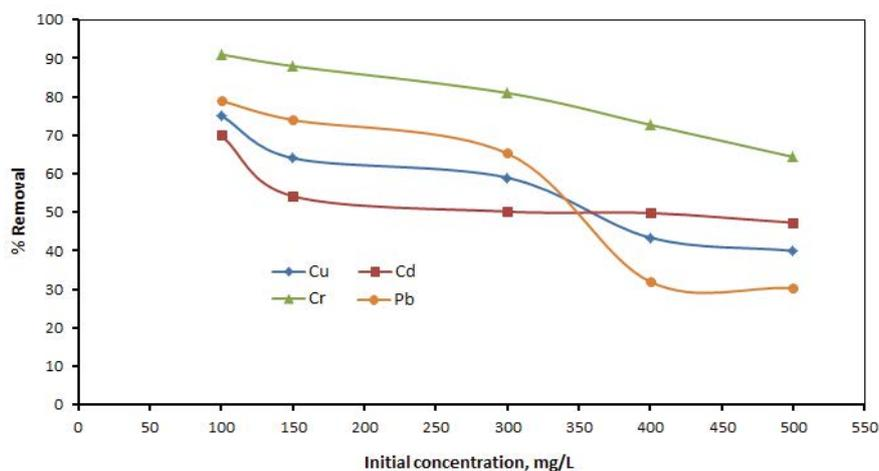
Fig. 7. Effect of initial concentration on the percentage removal of metal ions using potato peels. Experiment conditions: initial concentration, 100–500 mg/L; temperature, room temperature (25°C); adsorbent dose, 1 g; particle size, 250  $\mu$ m; shaking rate, 150 rpm, and pH, for Cd(II) pH = 6, for Cu(II), Pb(II) and Cr(III) pH = 4.
