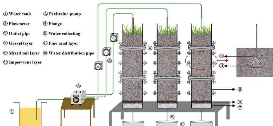
Fig. 2. SWIS simulation devices.
