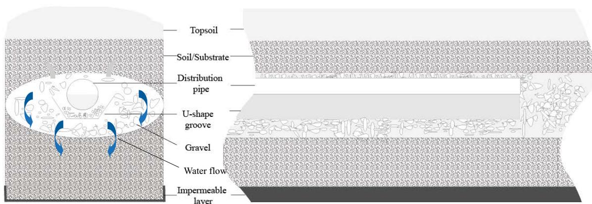
Fig. 1. Schematic diagram of subsurface wastewater infiltration system.
