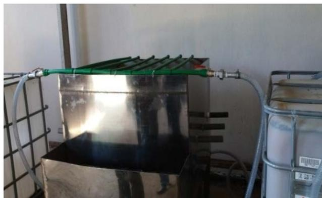
Fig. 4. Biobed system with an OOMWW tank on the right and a leaches collection tank on the left.
