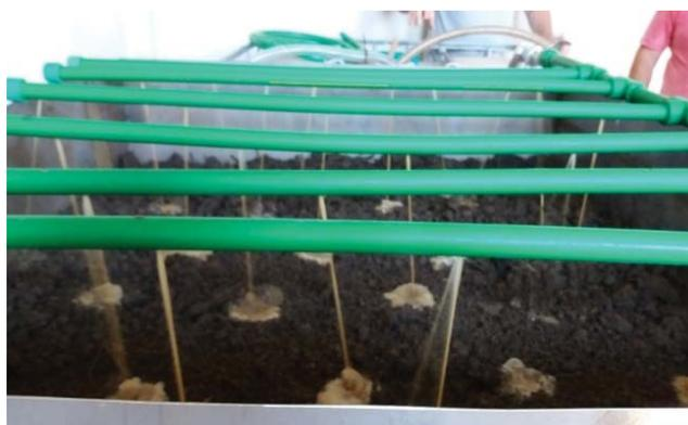
Fig. 3. Input of OOMWW into the biobed.
