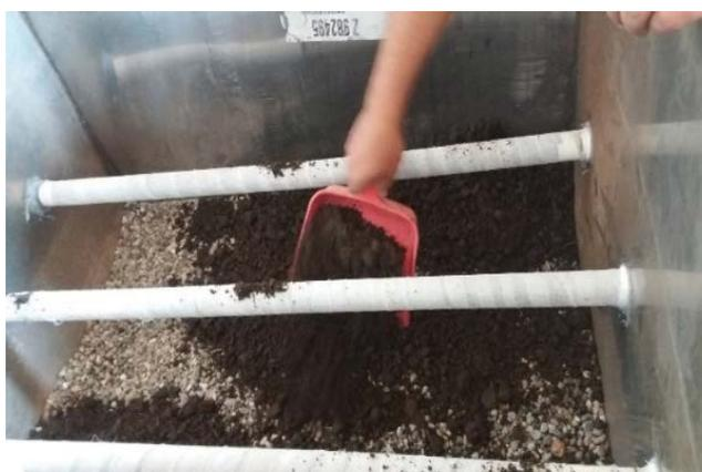
Fig. 2. Biomixture placement above the gravel.
