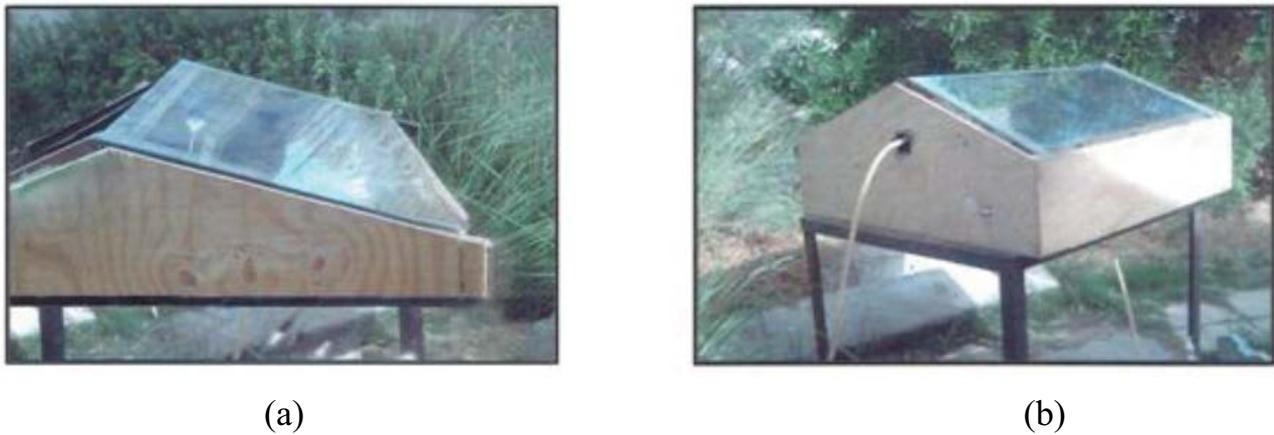
Fig. 1. Photographs of tested solar stills: (a) CSS and (b) EBSS.
