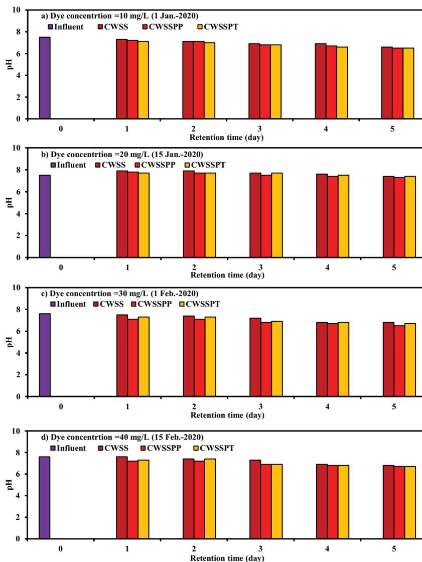
Fig. 2. Influent and effluent values of pH vs. the detention time in the unplanted and planted CW units packed with sewage sludge for different Congo red dye concentrations.
