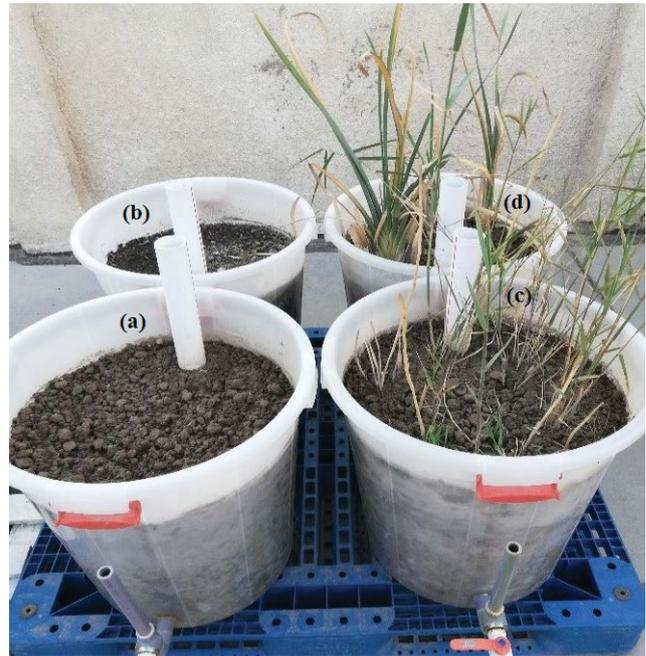
Fig. 1. Constructed wetland units manufactured in the present study (a & b) unplanted, (c) planted with *Phragmites australis* and (d) planted with *Typha domingensis*.
