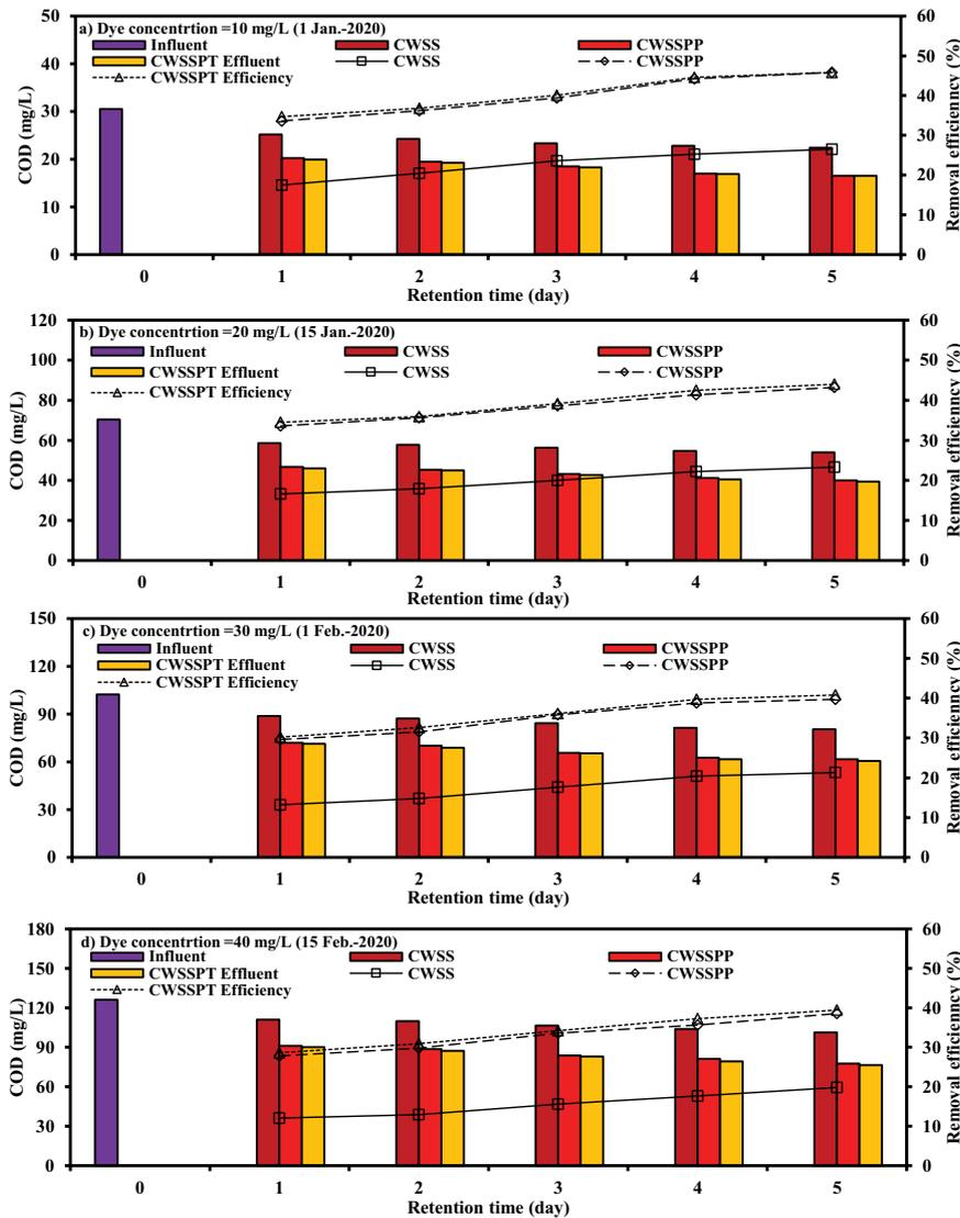
Fig. 3. Influent and effluent values of COD with removal efficiencies vs. the detention time in the unplanted and planted CW units packed with sewage sludge for different Congo red dye concentration.
