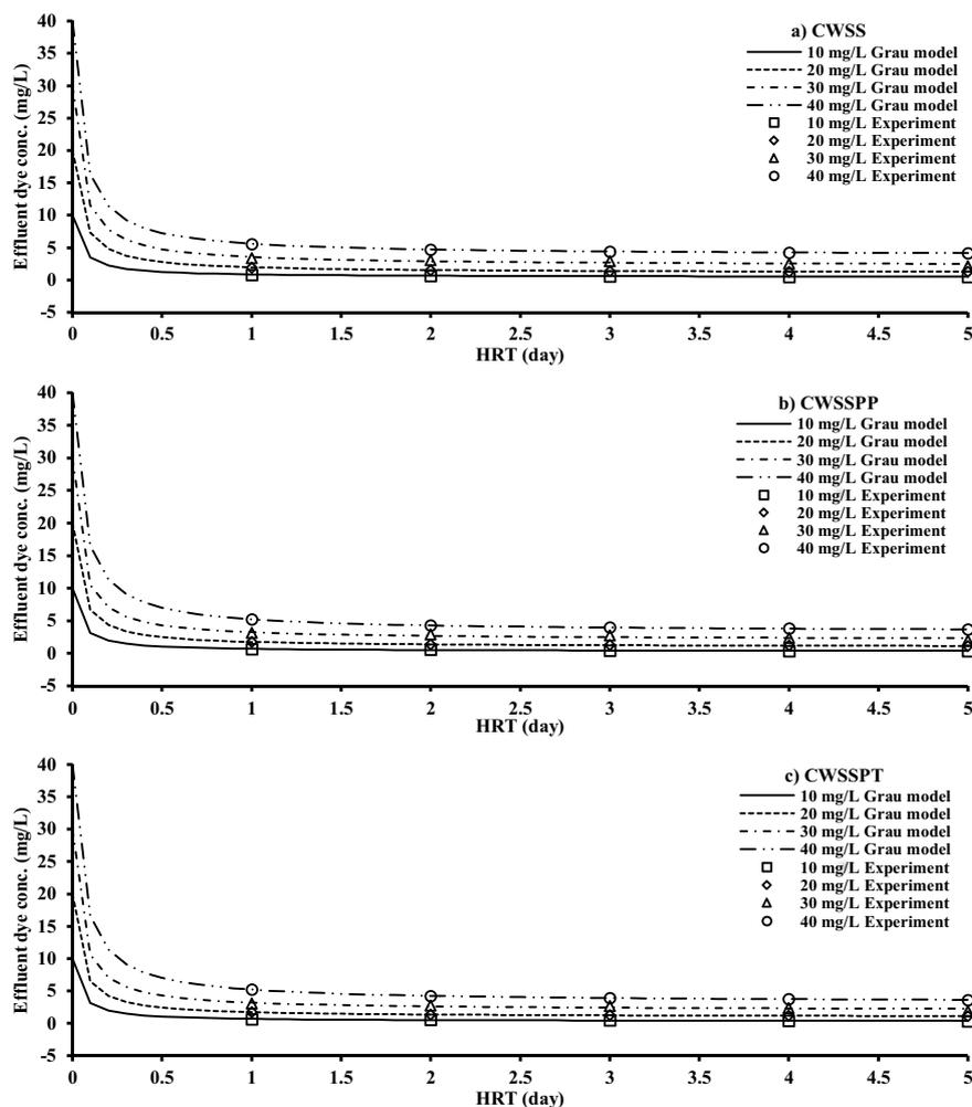
Fig. 7. Grau second-order kinetic model for effluent concentrations of Congo red dye in comparison with experimental measurements vs. the detention time in the unplanted and planted CW units packed with sewage sludge.
