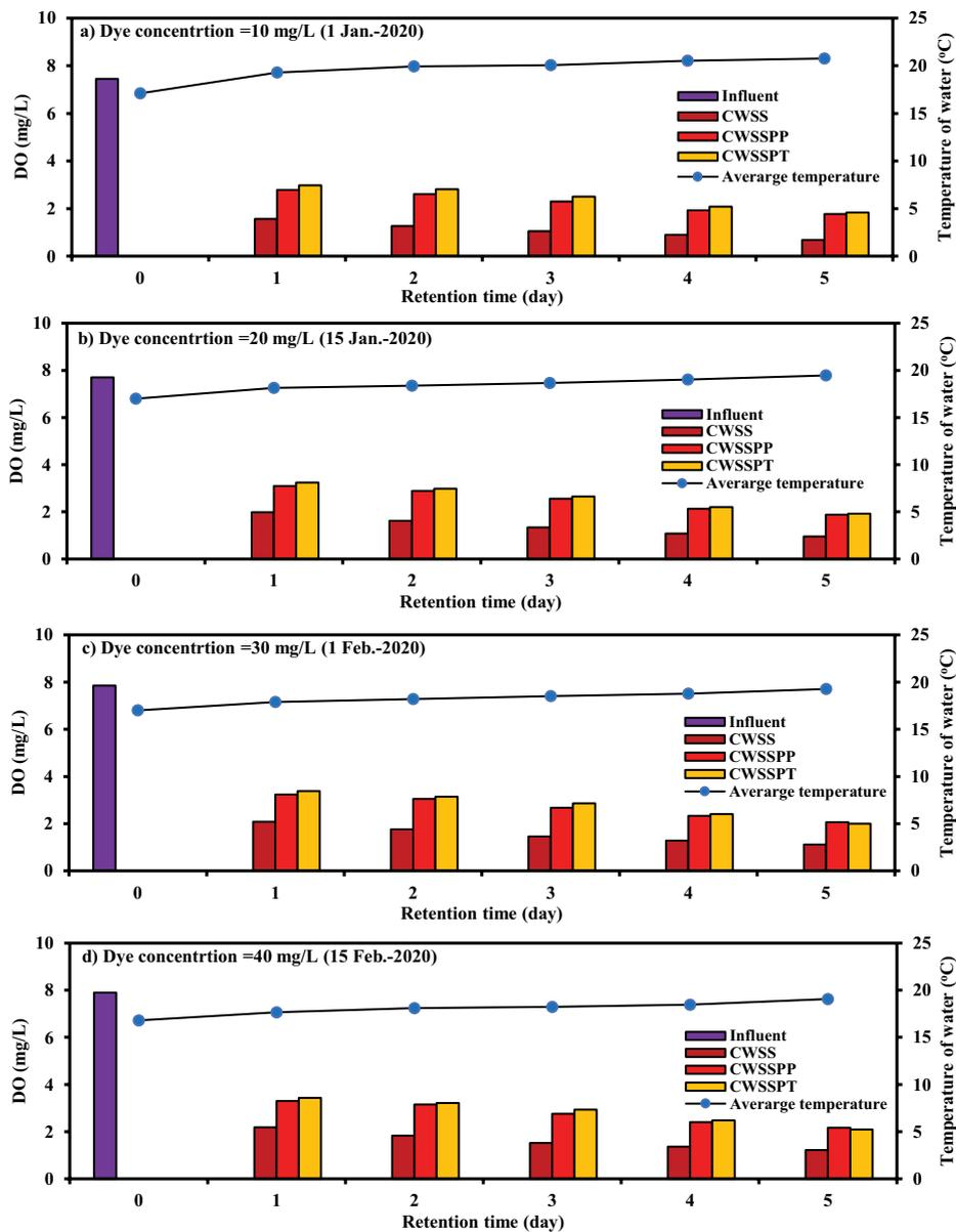
Fig. 4. Influent and effluent concentrations of DO with water temperature vs. the detention time in the unplanted and planted CW units packed with sewage sludge for different Congo red dye concentrations.
