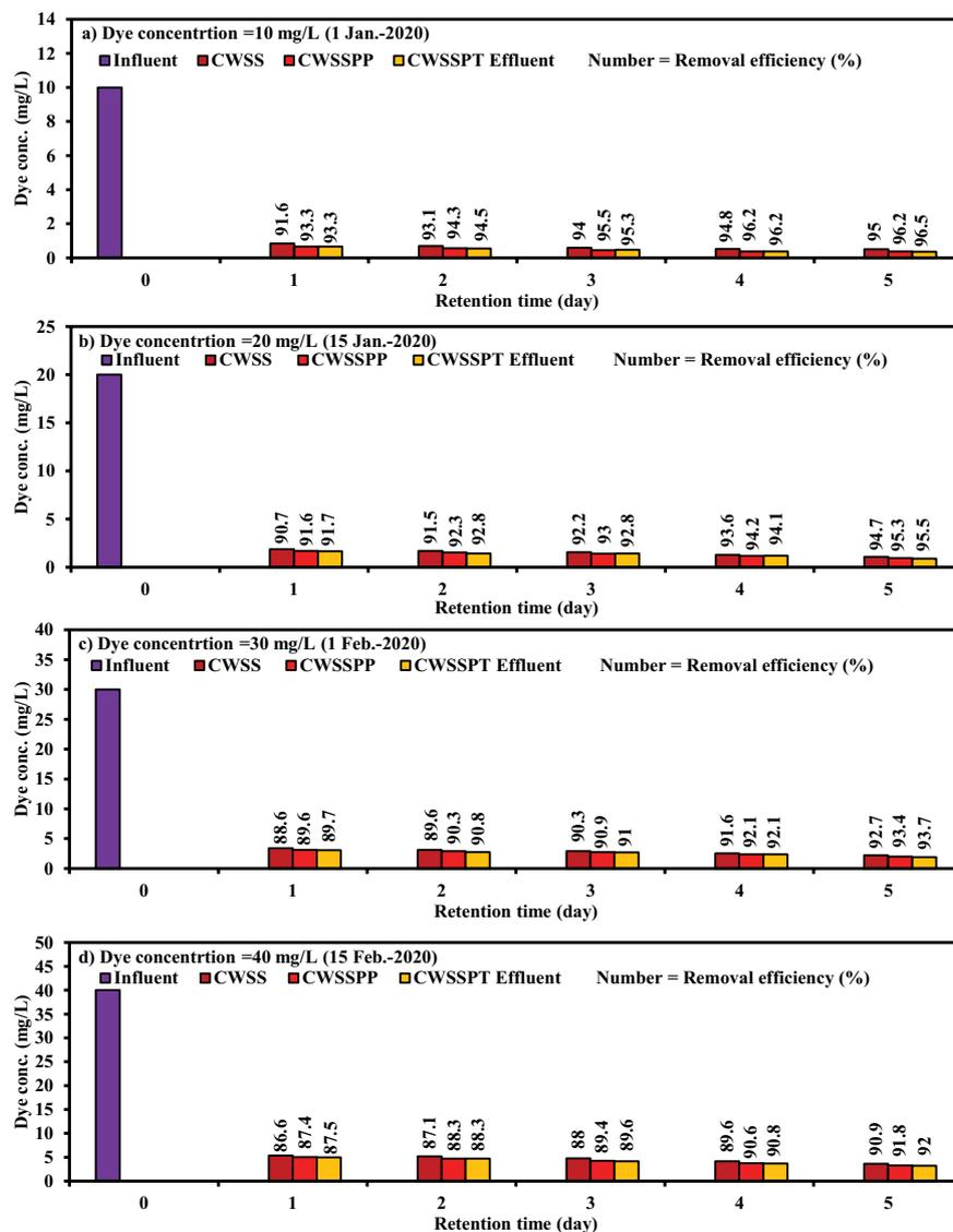
Fig. 5. Influent and effluent concentrations of Congo red dye with removal efficiencies vs. the detention time in the unplanted and planted CW units packed with sewage sludge.
