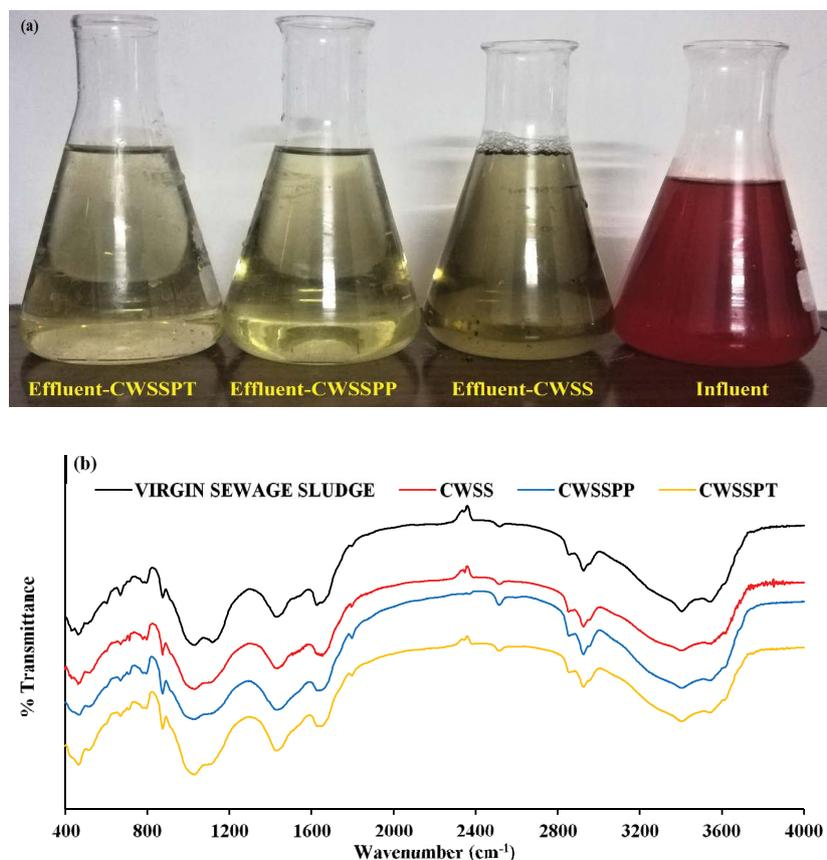
Fig. 6. (a) Appearance of influent and effluent wastewater treated by different CW units packed with sewage sludge after 5 d and influent dye concentration of 40 mg/L, (b) Infrared absorption spectrums for sewage sludge of unplanted and planted CWs units before and after sorption of Congo red dye.
