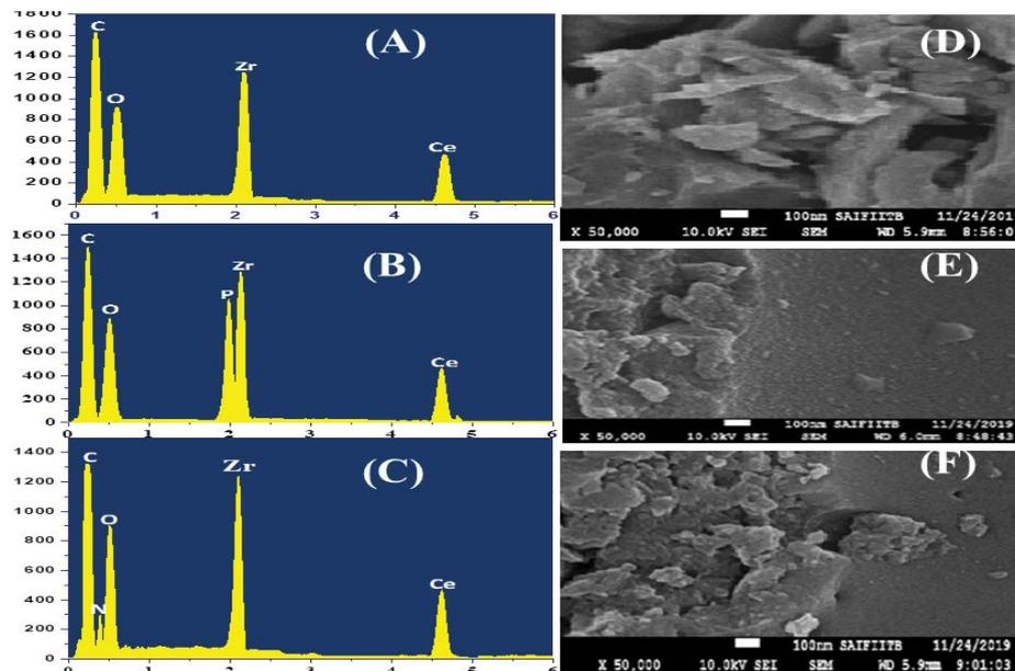
Fig. 5. EDX: (A) before, (B and C) after adsorption of  $\text{PO}_4^{3-}$  and  $\text{NO}_3^-$ ; FESEM: (D) before, (E and F) after adsorption of  $\text{PO}_4^{3-}$  and  $\text{NO}_3^-$ .
