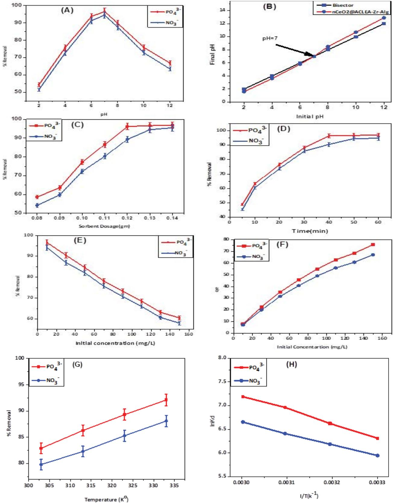
Fig. 6. (A) Effect of pH, (B) evaluation of  $pH_{zpc}$ , (C) effect of dosage, (D) effect of contact time, (E) effect of initial concentrations, (F) adsorption capacities,  $q_e$  vs. initial concentration, (G and H) effect of temperature.
