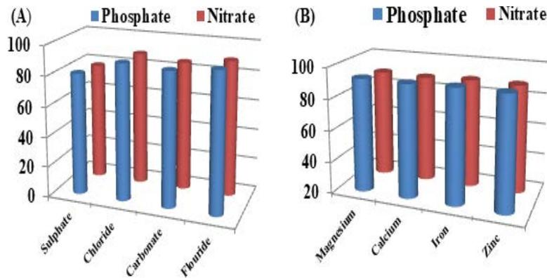
Fig. 9. Effect of interfering co-anions and co-cations, on % removal of phosphate and nitrate ions.
