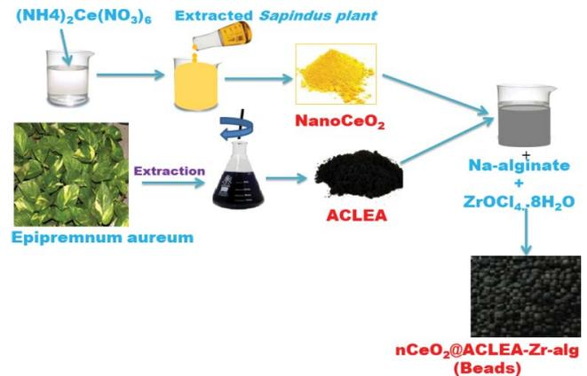
Fig. 2. Methodology for preparation of nCeO<sub>2</sub>@ACLEA-Zr-Alg -beads.
