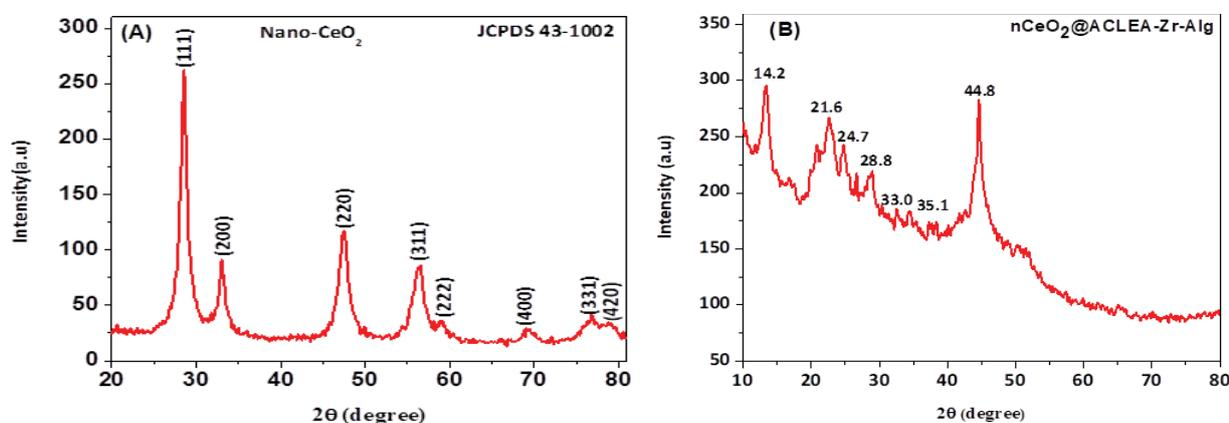
Fig. 3. XRD spectra of: (A) CeO<sub>2</sub> nanoparticles and (B) nCeO<sub>2</sub>@ACLEA-Zr-Alg'.
