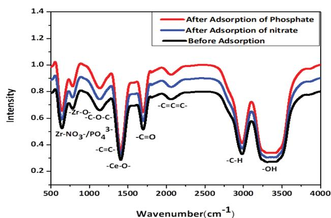
Fig. 4. FTIR spectra of before and after adsorption of NO<sub>3</sub><sup>-</sup> and PO<sub>4</sub><sup>3-</sup> ions.
