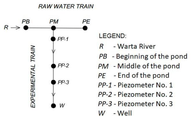
Fig. 1. Water flow scheme on the intake with measuring points.
