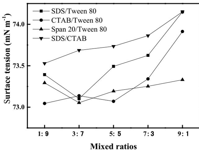
Fig. 2. Effect of surfactant mixtures on the surface tension of slurry.
