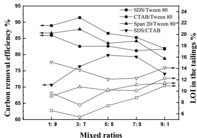
Fig. 1. Effects of mixed surfactants on decarburization performance.
