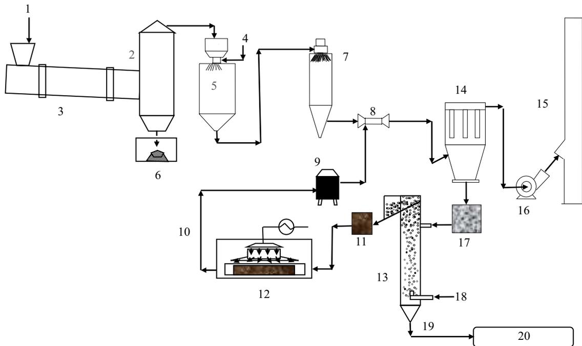
1—Medical waste; 2—Recombustion chamber; 3—Rotary kin; 4—Water; 5—Quench tower; 6—Bottom ash; 7—Semi-dry scrubber; 8—PAC injection; 9—PAC storage tank; 10—Pulverization; 11—The froths; 12—Microwave sintering furnace; 13—Flotation column; 14—Bag filter; 15—Stack; 16—Induced fan; 17—Raw fly ash; 18—Air; 19—Tailings; 20—Landfill disposal;
