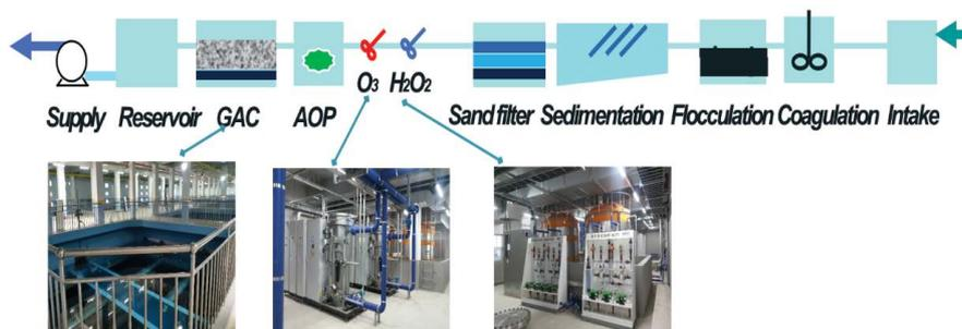
Fig. 2. Process of water treatment plant as a testbed.
