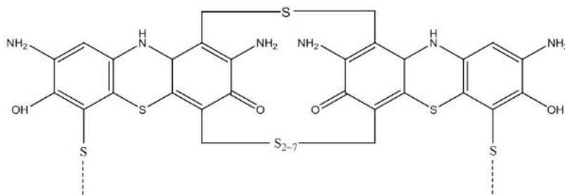
Fig. 1. Sulfur black molecular structure.
