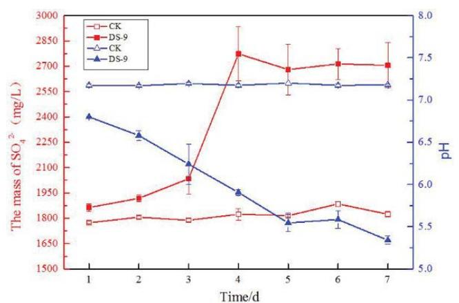
Fig. 6. The SO<sub>4</sub><sup>2-</sup> and pH change curves of DS-9 were continuously cultured for 7 d in the optimized degradation system.
