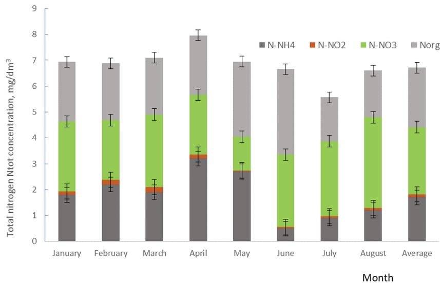
Fig. 7. Average monthly total nitrogen  $N_{tot}$  concentrations taking into account mineral and organic components in purified wastewater during the period from January to August 2020.
