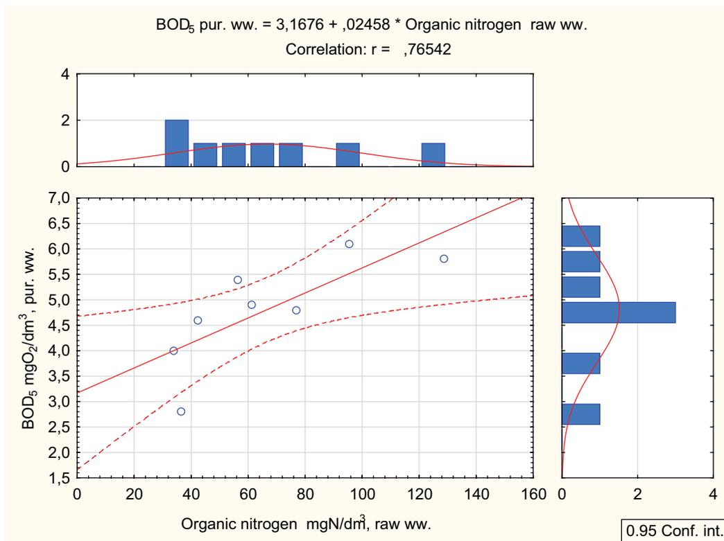
Fig. 9. Categorized scatter plot with regression line for  $BOD_5$  indicator in purified wastewater and organic nitrogen  $N_{org}$  in raw wastewater. The correlation was tested for the monthly average.
