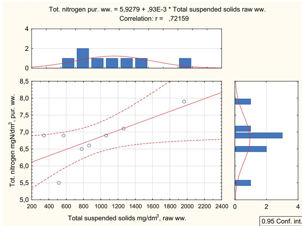
Fig. 10. Categorized scatter plot with regression line for total nitrogen  $N_{tot}$  in purified wastewater and total suspended solids TSS in raw wastewater. The correlation was tested for the monthly average.
