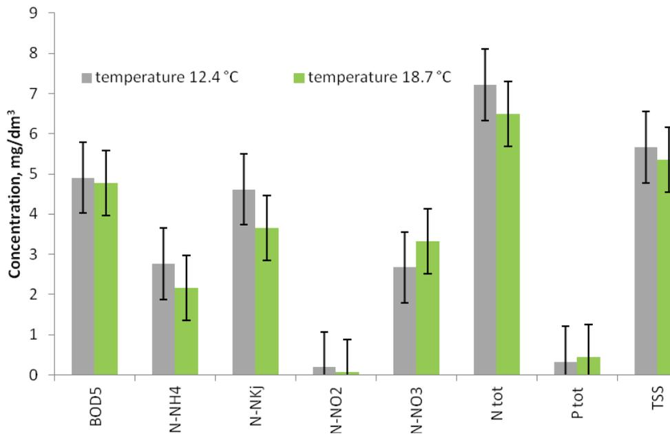
Fig. 3. Average concentration of selected quality indicators of purified wastewater within the researched period depending on the average wastewater temperature.
