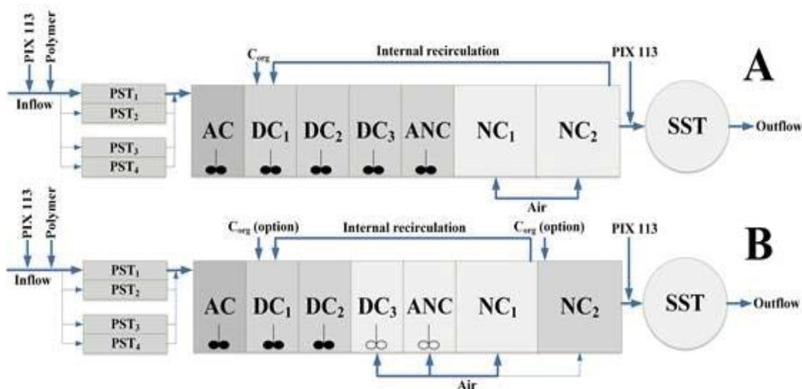
Fig. 1. Wastewater treatment plant before (A) and after (B) modification diagram: AC – anaerobic chamber, DC<sub>n</sub> and ANC – anoxic chambers, NC<sub>n</sub> – oxic chamber (nitrification), PST<sub>n</sub> – pre-settlement tanks, SST – secondary settlement tank.
