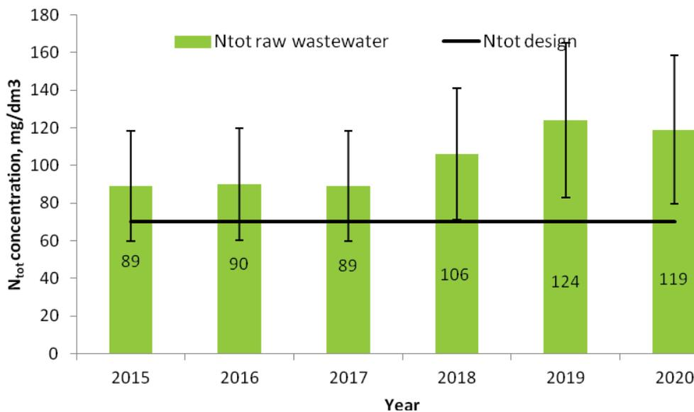
Fig. 4. Annual average total nitrogen  $N_{tot}$  concentrations in raw wastewater during 2015–2020 period versus the designed value amounting to 70 mg/dm<sup>3</sup>.
