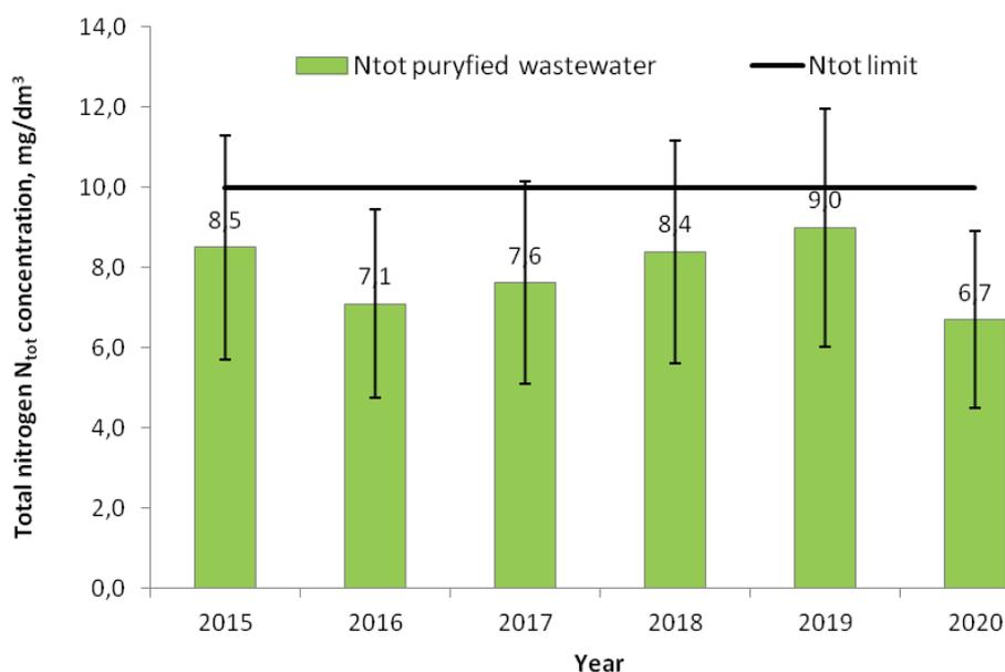
Fig. 5. Annual average total nitrogen N<sub>tot</sub> concentrations in purified wastewater from 2015 to August 2020.
