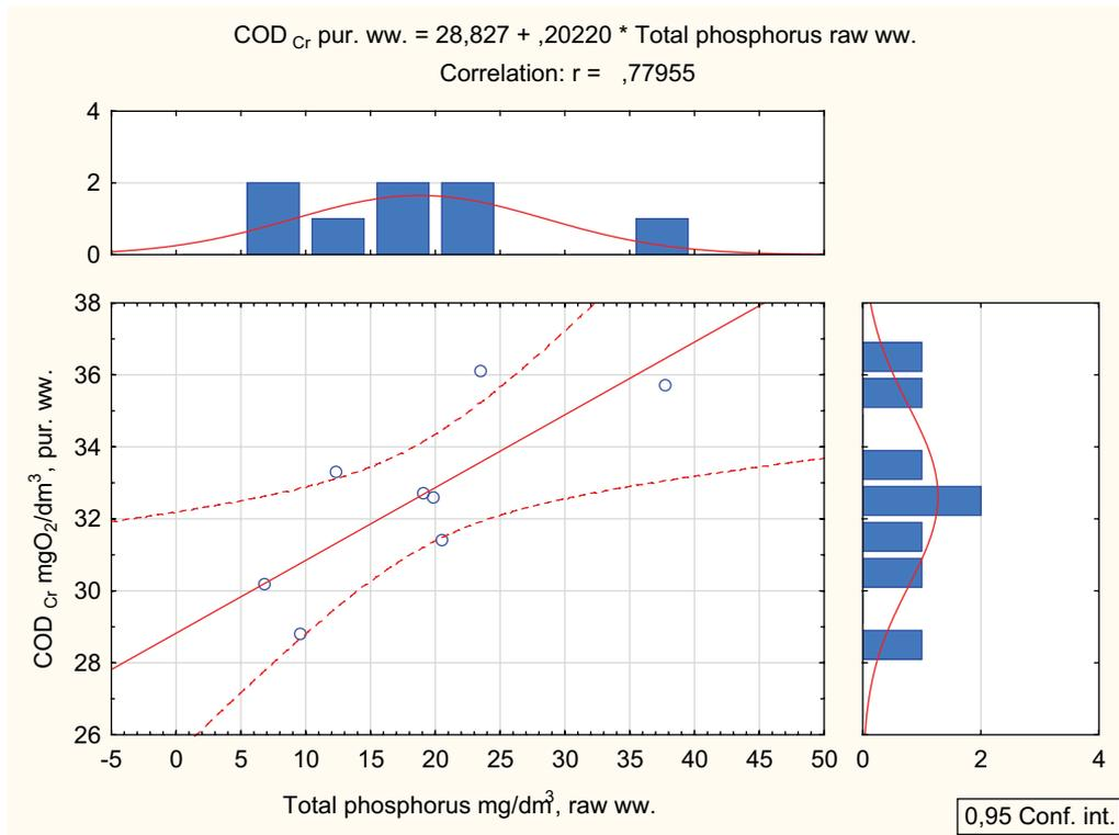
Fig. 8. Categorized scatter plot with regression line for  $COD_{Cr}$  indicator in purified wastewater and total phosphorus  $P_{tot}$  in raw wastewater. The correlation was tested for the monthly average.
