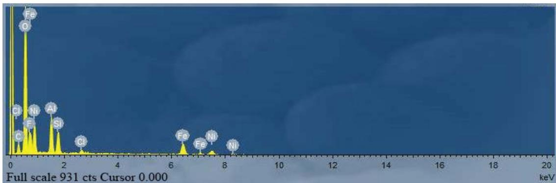
Fig. 3. EDS pattern of FAN composite oxide after adsorption.
