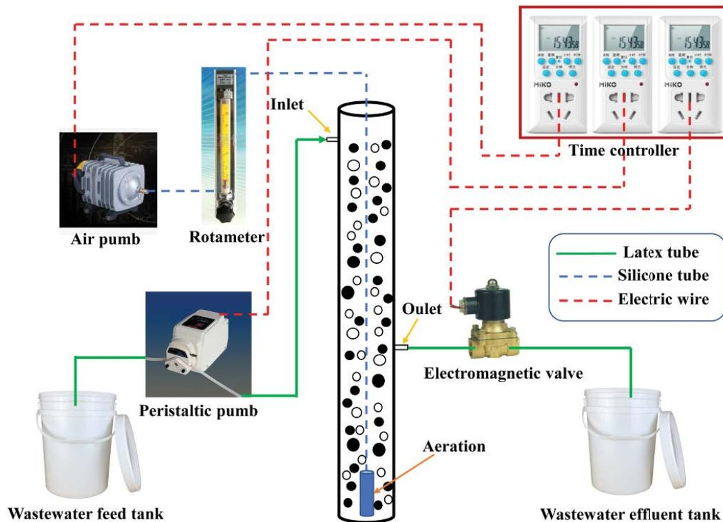
Fig. 1. Experimental setup of the aerobic granular sequencing batch reactor.
