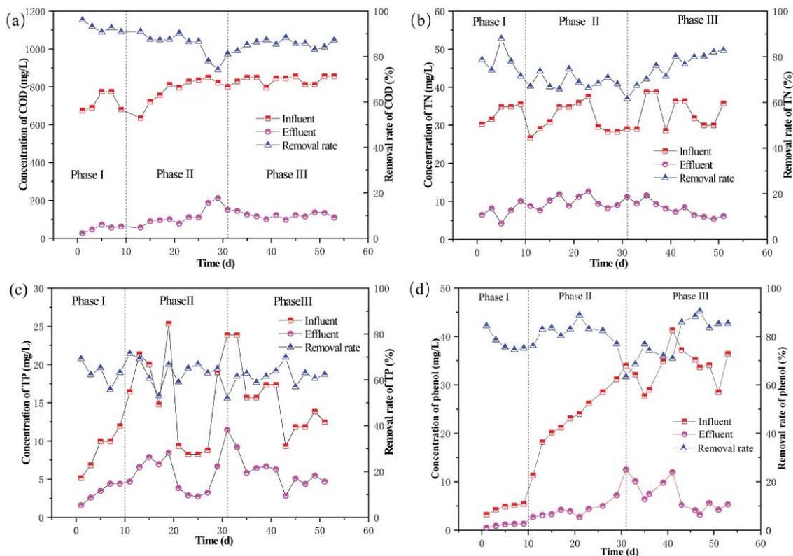
Fig. 3. The pollutant removal performance of the AGSBR during operation: (a) COD, (b) TN, (c) TP, and (d) phenol removal.
