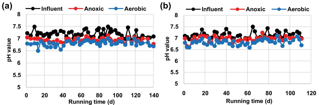
Fig. 13. Variation of pH with time for (a) non-coated and (b) coated media.
