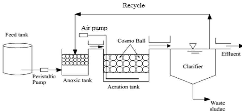
Fig. 2. Illustration of the laboratory-scale cosmoball system.
