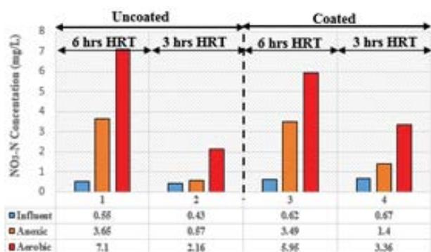
Fig. 10. Nitrate concentration under feeding, anoxic and aerobic conditions when coated and non-coated media were used at HRT of 6 and 3 h.
