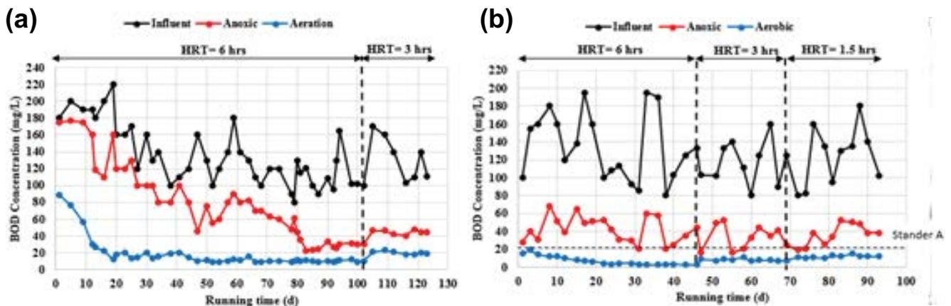
Fig. 4. BOD<sub>5</sub> concentration vs. time for (a) non-coated cosmoball and (b) coated cosmoball.
