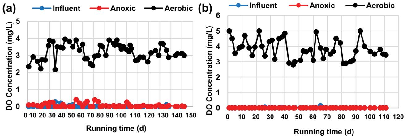
Fig. 12. DO concentration for (a) non-coated and (b) coated media.
