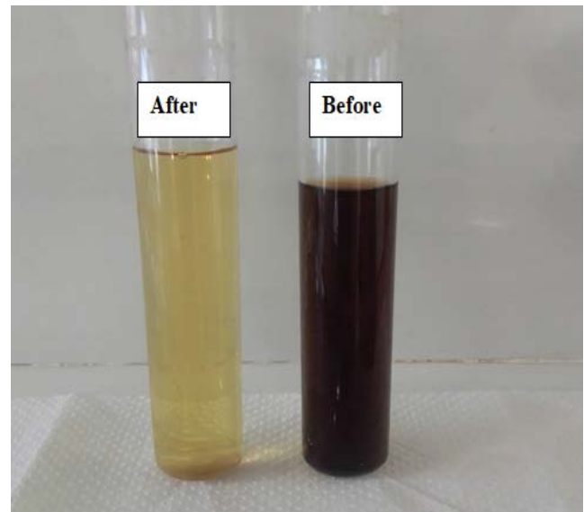
Fig. 5. Leachate before and after pretreatment.
