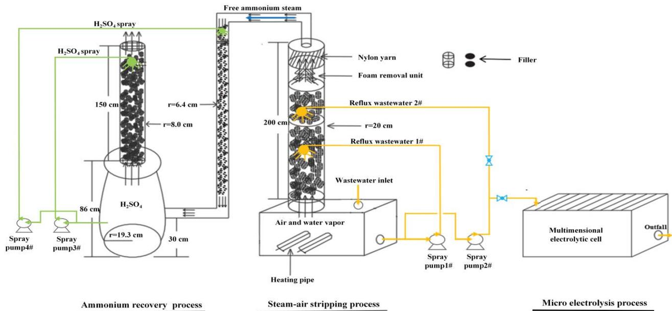
Fig. 1. Micro-electrolysis combined with steam-air stripping process equipment.
