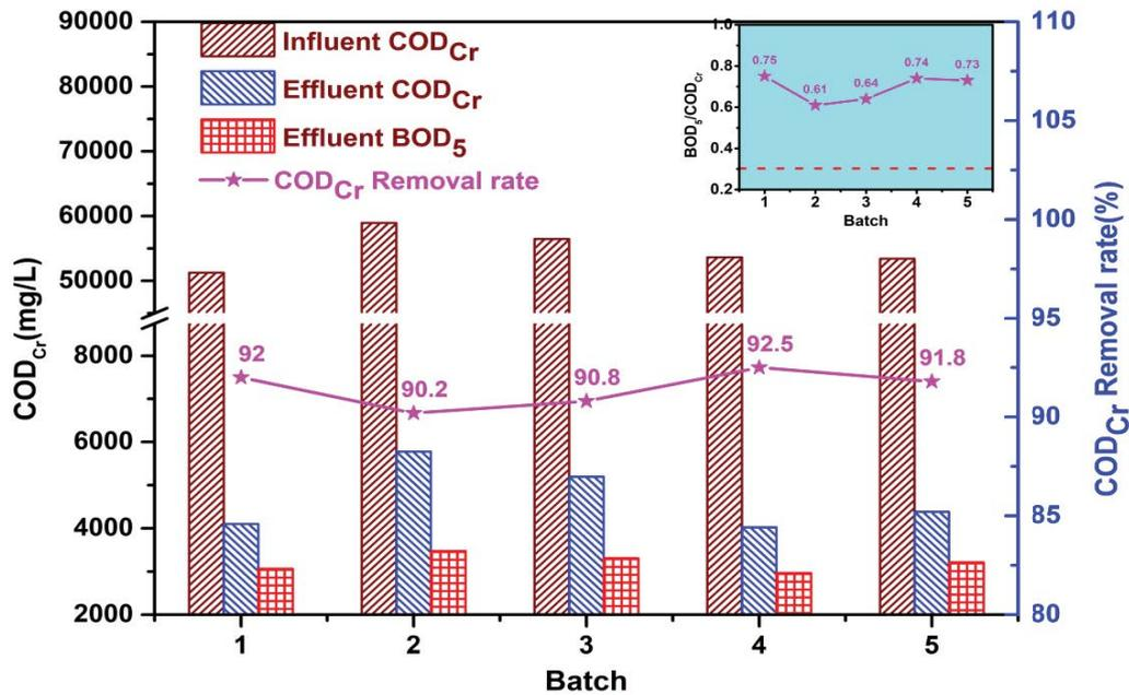
Fig. 7. The removal efficiency trends of COD<sub>Cr</sub> in the destructive experiments of the micro-electrolysis process.
