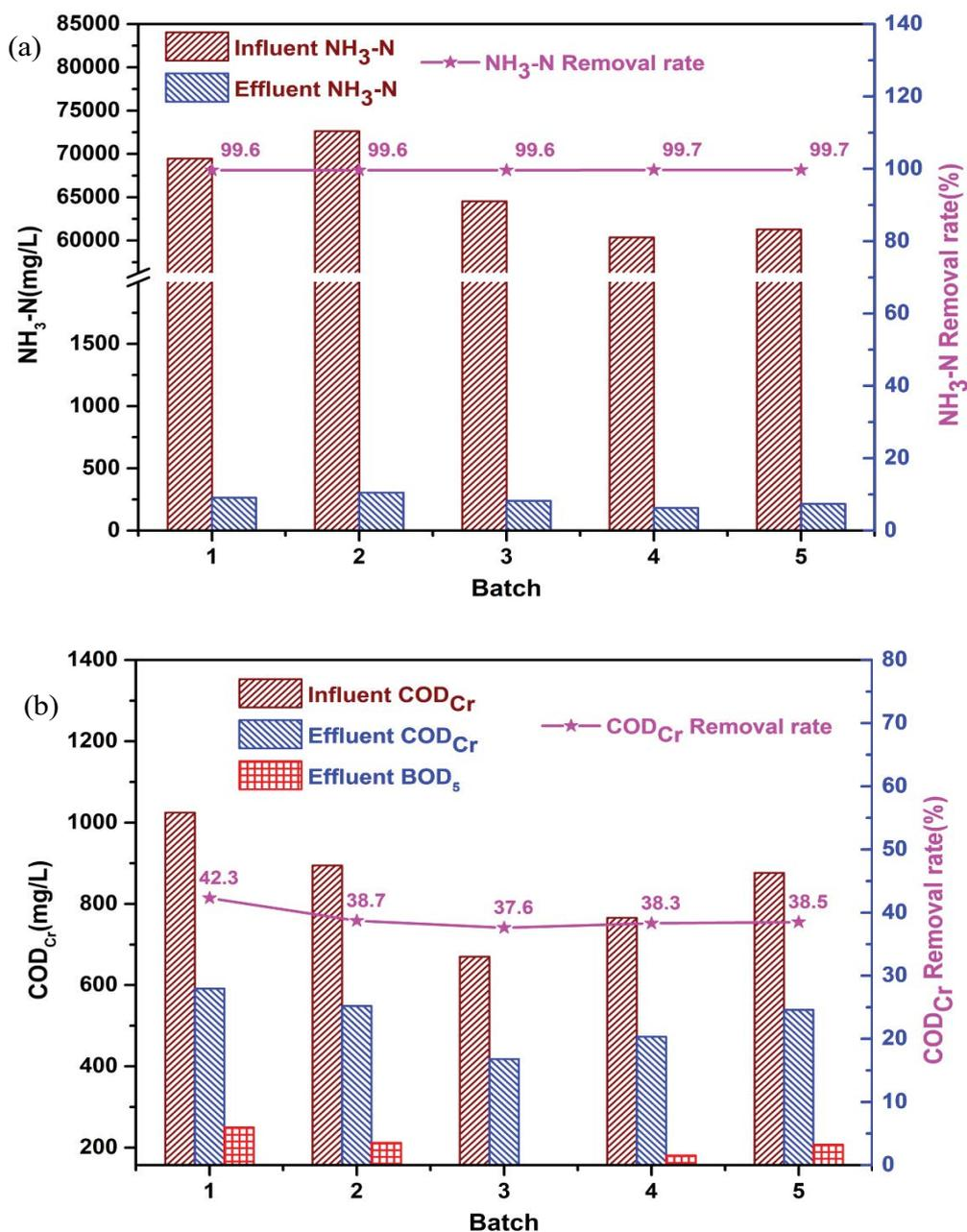
Fig. 6. The removal efficiency trends of NH<sub>3</sub>-N (a) and COD<sub>Cr</sub> (b) in the destructive experiments of steam-air stripping process.
