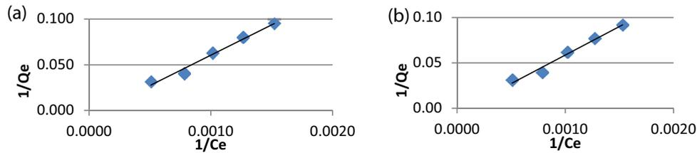
Fig. 14. Langmuir isotherm after adsorption on clay soil (a) and on cactus (b).
