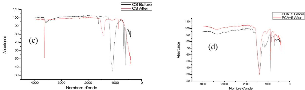
Fig. 6. Evolution of the infrared bands of clay soil (c) and activated carbon powder + sand (d) before and after adsorption.
