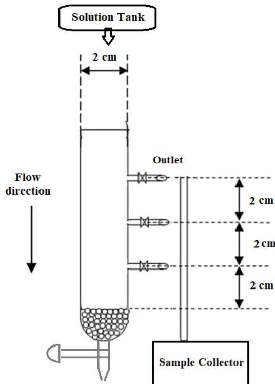
Fig. 4. Fixed bench support for experiments.
