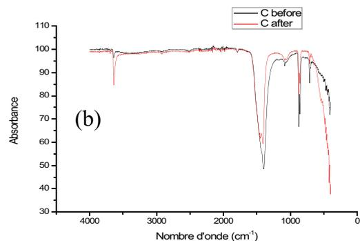
Fig. 5. Evolution of infrared bands before and after adsorption for sawdust (a) cactus (b).
