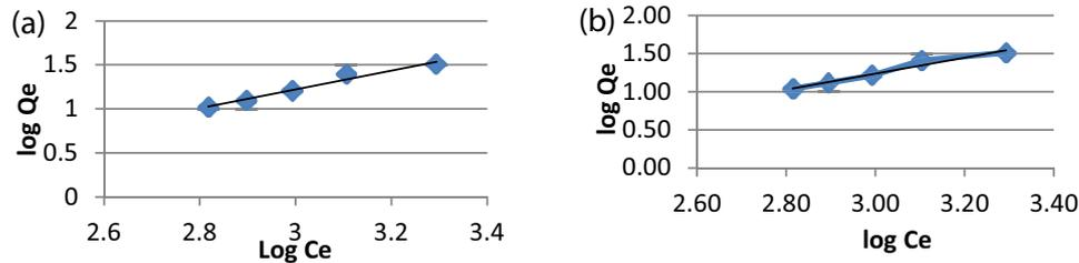
Fig. 15. Freundlich isotherm after adsorption on clay soil (a) and on cactus (b).
