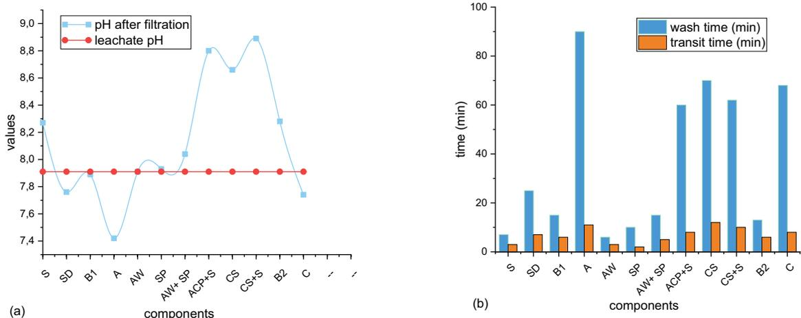
Fig. 8. (a) Evolution of the pH after filtration and (b) evolution of the transit time and filtration.
