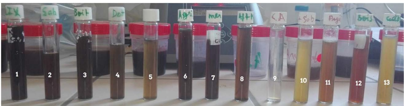
Fig. 7. Visual appearance of filtrates from different matrices: 1: leachate; 2: sand (S); 3: sawdust (B1); 4: core of dates (CD); 5: fruit of the Casuarina tree (A); 6: agricultural waste (AW); 7: sea plant (SP); 8: agricultural waste + sea plant; 9: activated carbon powder + sand; 10: clay soil (CS) + sand; 11: clay soil (CS); 12: sawdust (B2); 13: cactus (C).
