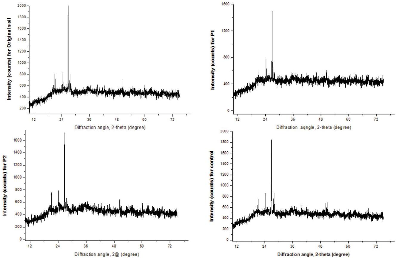
Fig. 4. XRD analysis of before-treated dried original soil, after-treated dried soil from *Cyperus ustulatus* plant (P1) in CW, *Typha latifolia* plant (P2) in CW, and without plant (control) in CW, respectively.
