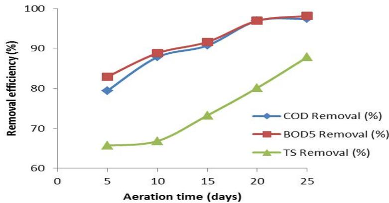
Fig. 2. Effect of aeration days on the efficiency of constructed wetland in the removal of COD, BOD<sub>5</sub> and TS.
