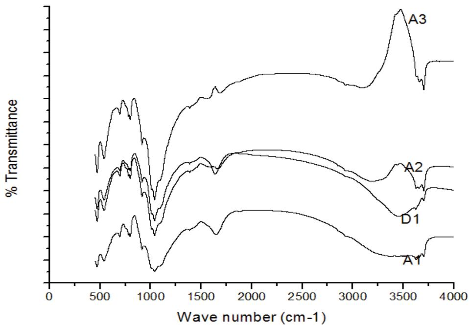
Fig. 5. FTIR spectra soil (D1) before treated dried original soil, (A1) after treated dried soil with *Cyperus ustulatus* (P1), (A2) after treated dried soil with *Typha latifolia* (P2), and (A3) after treated dried soil without plant (control).
