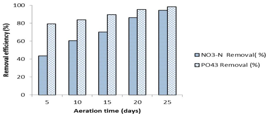
Fig. 3. The removal efficiency of nutrients in various days of aeration with wetland treatment.
