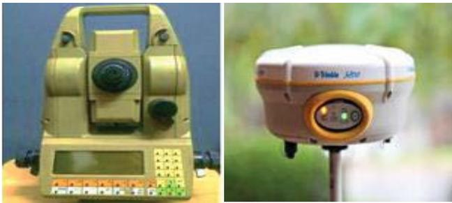
Fig. 3. Monitoring instruments (the figure on the left shows Leica TC402 Precision Total Station, and the figure on the right shows HD5800 Static GPS Receiver).
