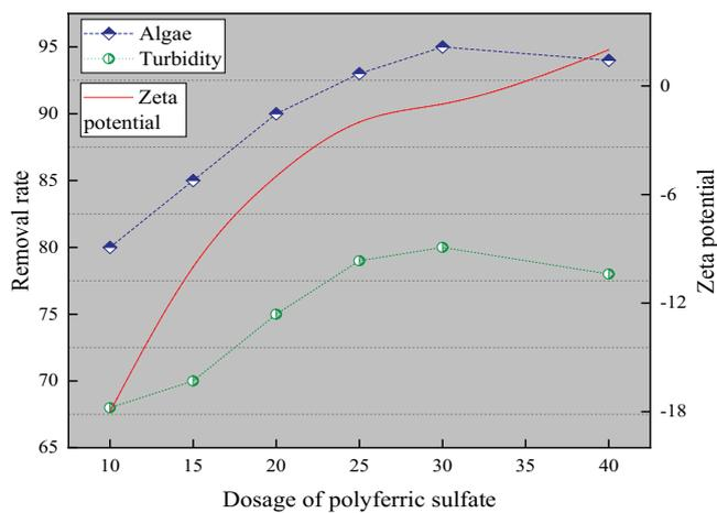
Fig. 2. Effect of different content of polyferric sulfate on the water body.
