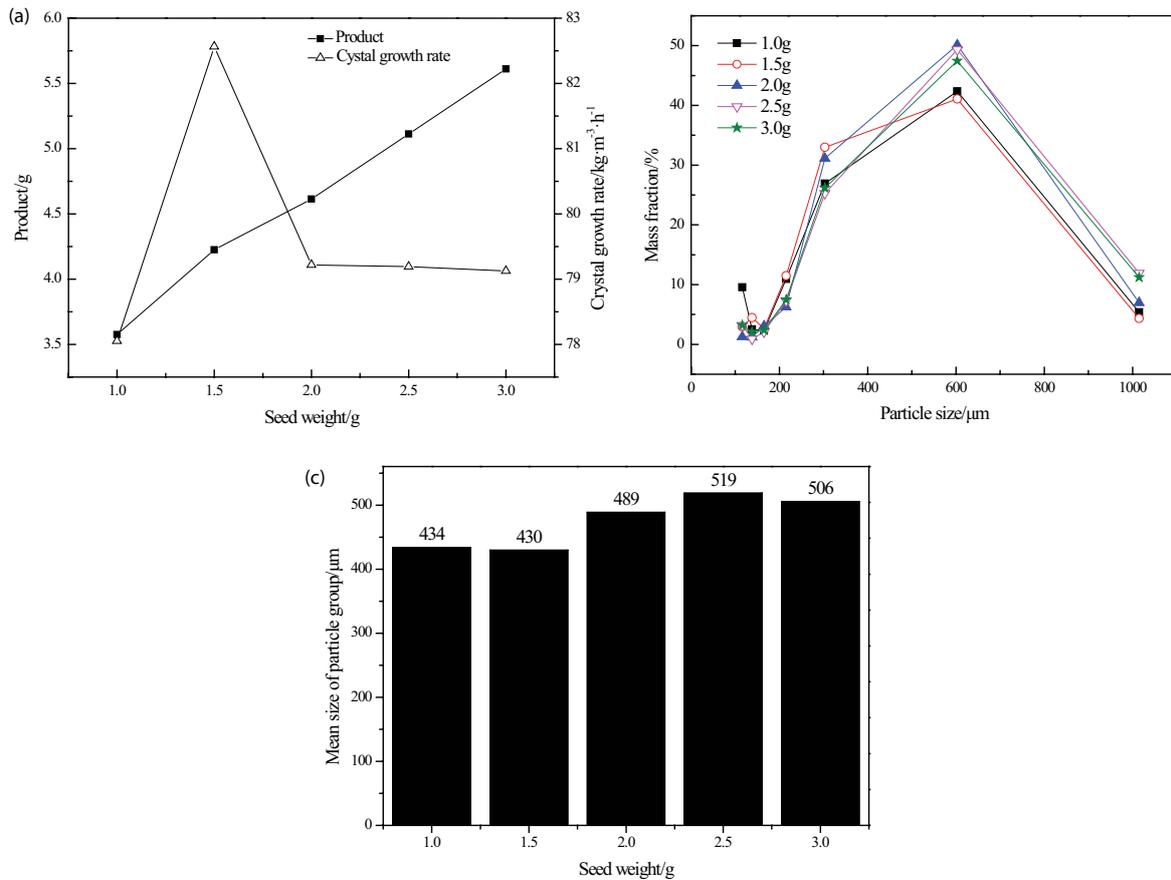
Fig. 9. Impact of seed weight on (a) product and crystal growth rate, (b) particle size distribution and (c) mean size of 1,2-diphenylethane.
