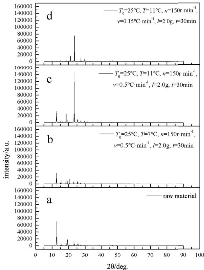
Fig. 10. X-ray power diffraction pattern of 1,2-diphenylethane.
