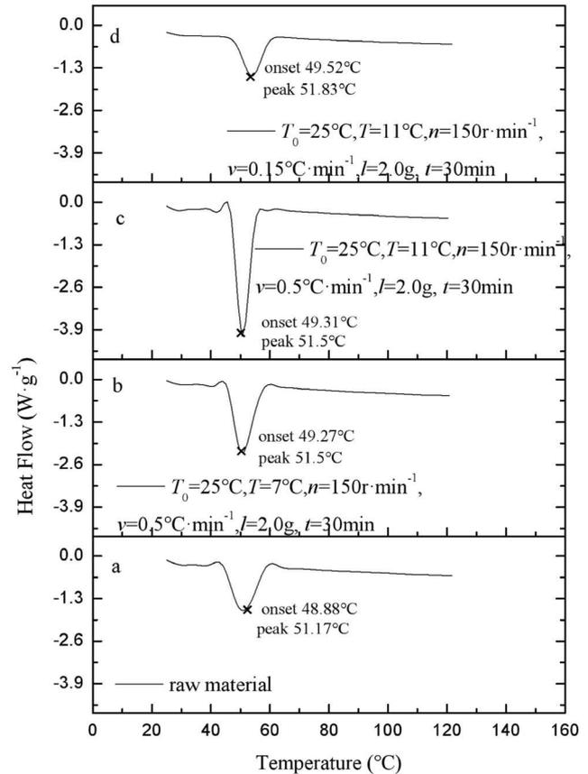
Fig. 11. DSC of 1,2-diphenylethane.
