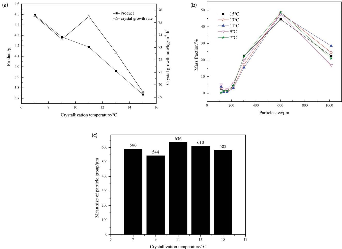
Fig. 4. Impact of crystallization temperature on (a) product and crystal growth rate, (b) particle size distribution, and (c) mean size of 1,2-diphenylethane.
