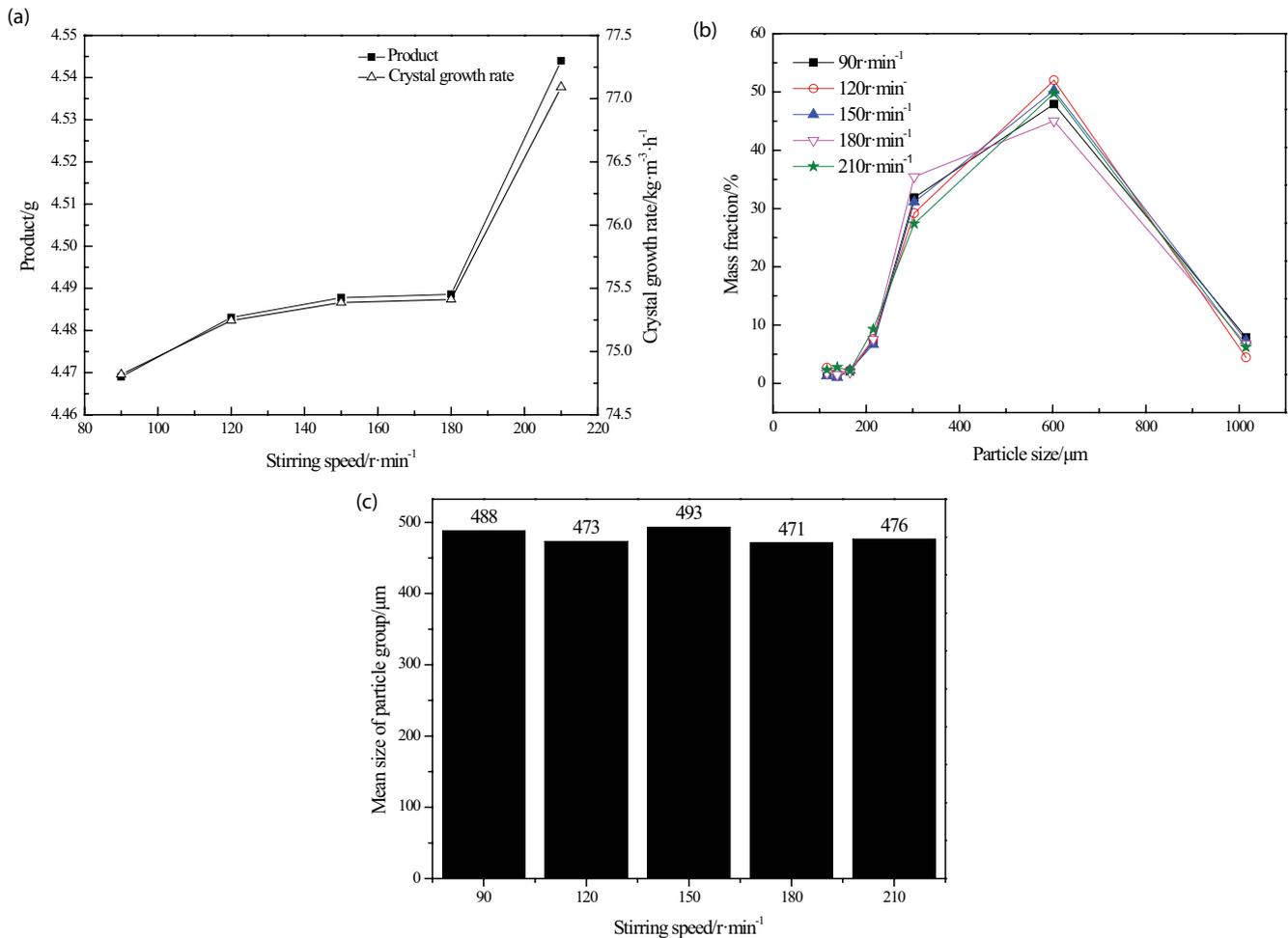
Fig. 7. Impact of stirring speed on (a) product and crystal growth rate, (b) particle size distribution and (c) mean size of 1,2-diphenylethane.
