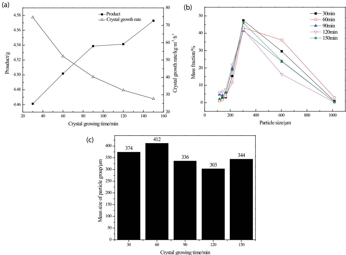
Fig. 5. Impact of crystal growing time on (a) product and crystal growth rate, (b) particle size distribution and (c) mean size of 1,2-diphenylethane.
