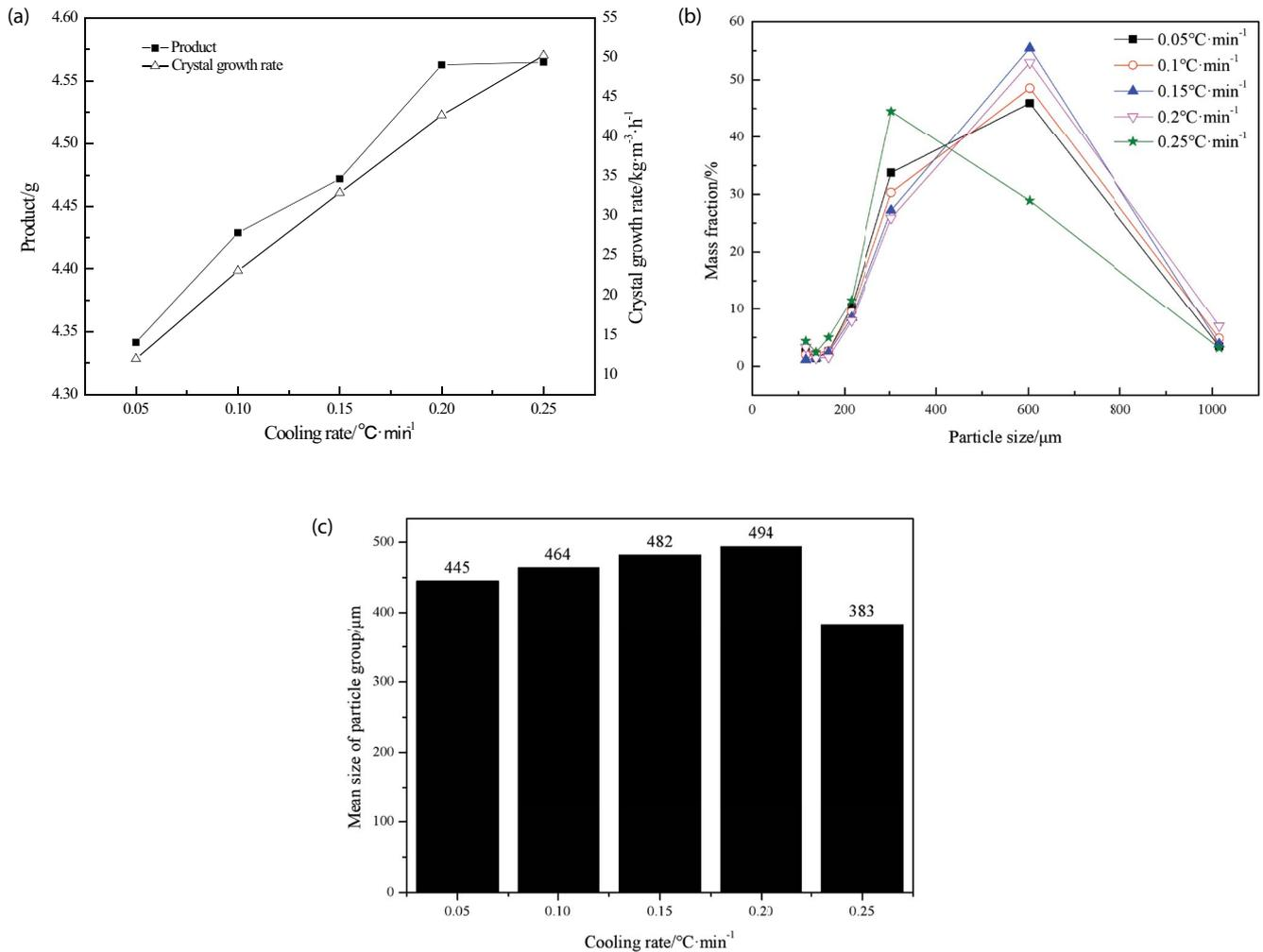
Fig. 6. Impact of cooling rate on (a) product and crystal growth rate, (b) particle size distribution and (c) mean size of 1,2-diphenylethane.
