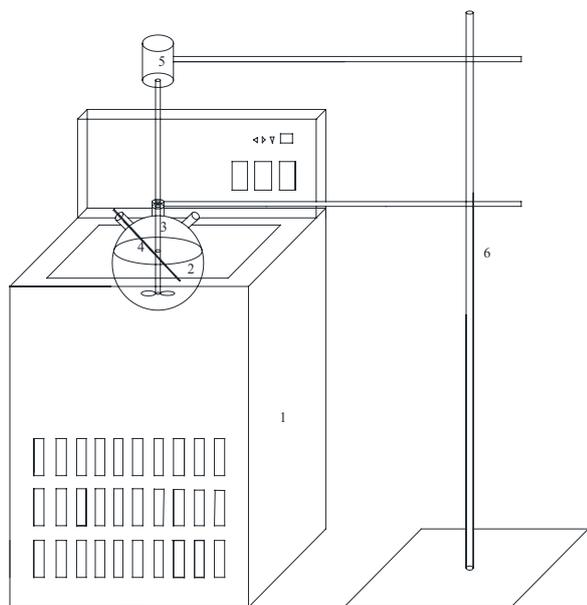
Fig. 3. The crystallization process of 1,2-diphenylethane. (1) Super thermostatic bath, (2) MSMPR crystallizer, (3) mechanical agitator, (4) thermometer, (5) motor, (6) iron support.
