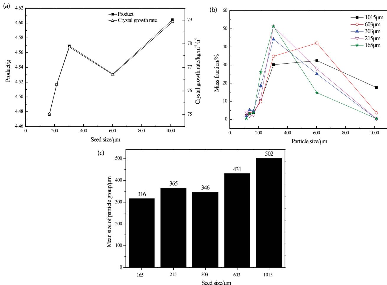
Fig. 8. Impact of seed size on (a) product and crystal growth rate, (b) particle size distribution and (c) mean size of 1,2-diphenylethane.
