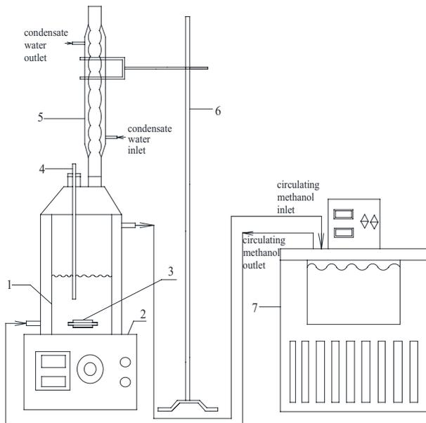
Fig. 2. Schematic diagram of determining solubility of 1,2-diphenylethane. (1) Jacketed vessel, (2) magnetic stirrer, (3) stir bar, (4) thermometer, (5) condenser, (6) iron support, (7) super thermostatic bath.
