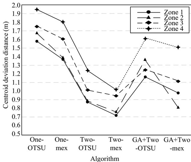
Fig. 6. Comparison of centroid deviation distance of different segmentation algorithms in wastewater pollution image processing.
