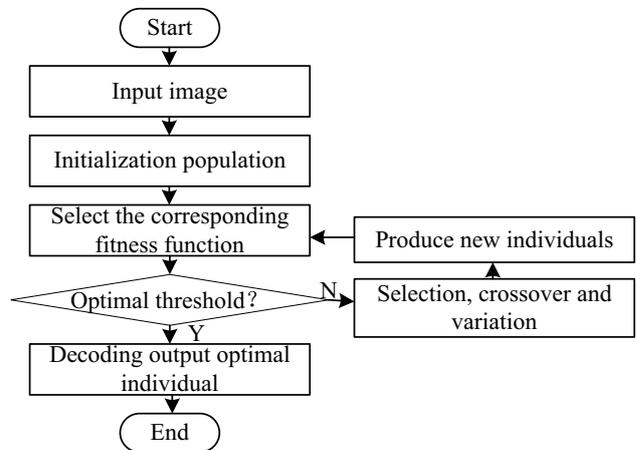
Fig. 2. Flow chart of two dimensional threshold image segmentation algorithm based on genetic algorithm.
