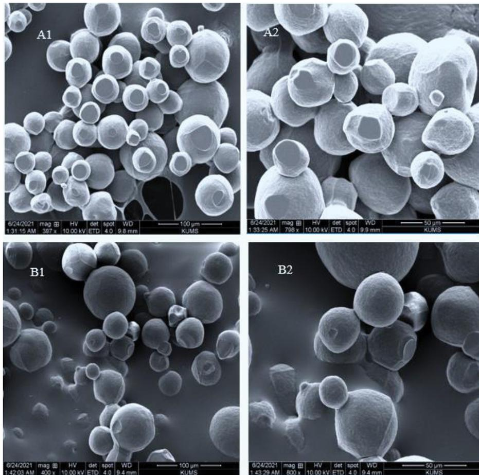
Fig. 4. Representative SEM images of sepharose beads at different magnifications: before immobilization (A1 and A2), after immobilization (B1 and B2).
