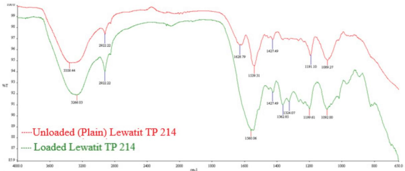
Fig. 10. FTIR spectrum of unloaded (plain) and loaded Lewatit TP 214.
