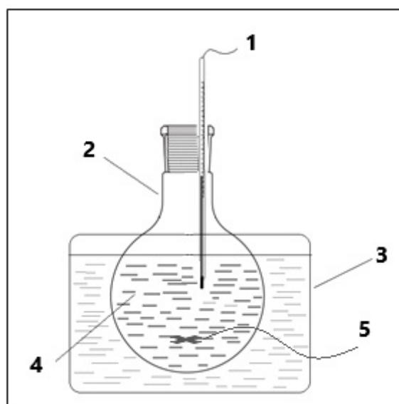
Fig. 1. Experimental setup: 1. Electronic thermometer, 2. Glass boiling flask, 3. Water bath, 4. Solution, 5. Magnetic stirring bar.
