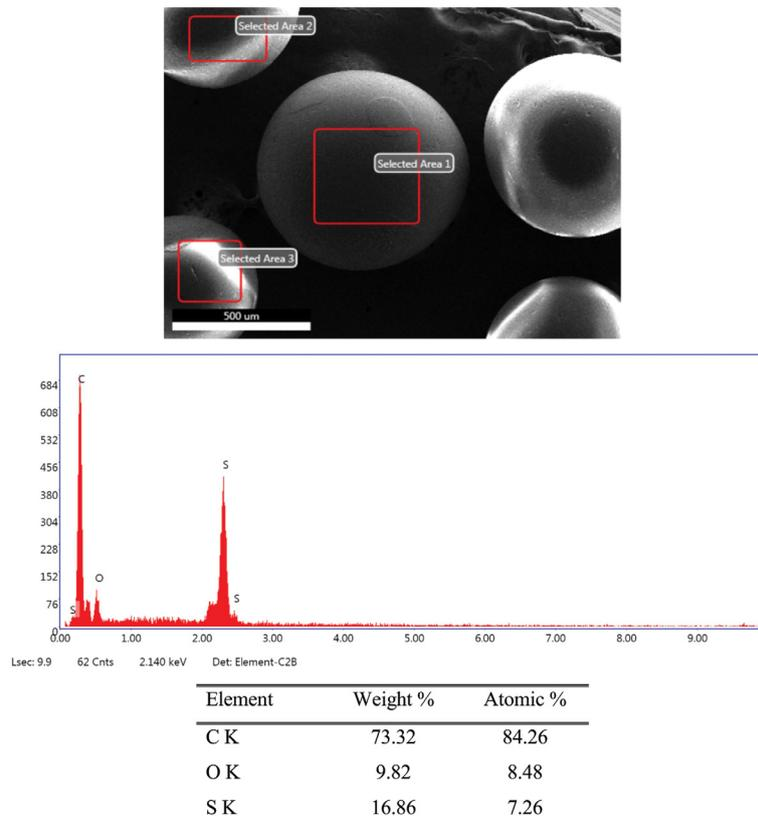
Fig. 11. SEM and EDS analysis of the Lewatit TP 214 commercial resin as-taken, before adsorption.
