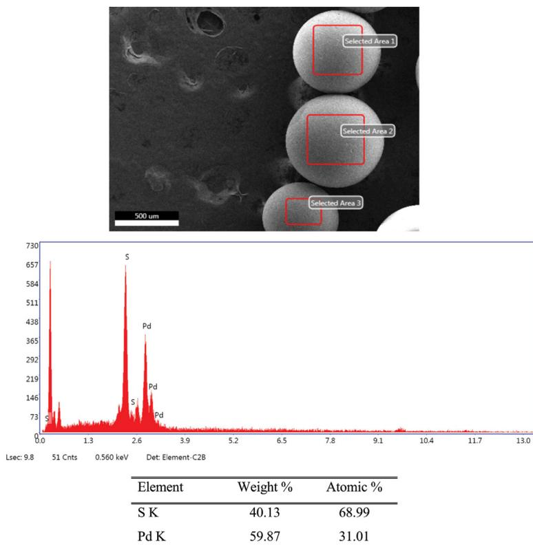
Fig. 12. SEM and EDS analysis of the Lewatit TP 214 commercial resin after Pd(II) adsorption.
