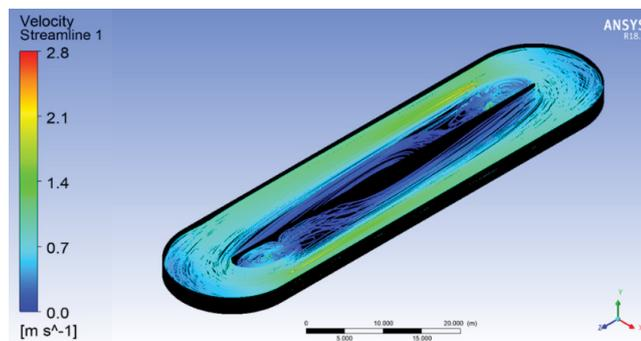
Fig. 14. Streamline velocity in the horizontal section of the oxidation ditch tank at impeller thrust of 2800 N.
