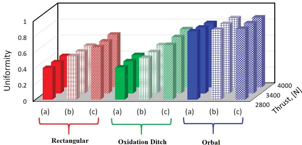
Fig. 21. The flow uniformity for cross-sections (a), (b), and (c) for the three tank geometries at different impeller thrusts
