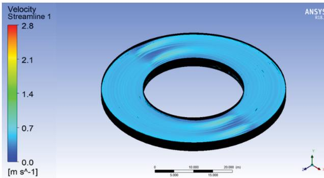
Fig. 17. Streamline velocity in the horizontal section of the orbal tank at impeller thrust of 2800 N.
