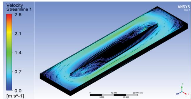
Fig. 11. Streamline velocity in the horizontal section of the rectangular tank at impeller thrust of 2800 N.
