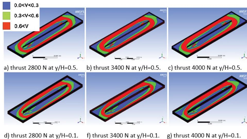
Fig. 10. Velocity contour of the rectangular bioreactor in the horizontal section at different height and different impeller thrust forces.
