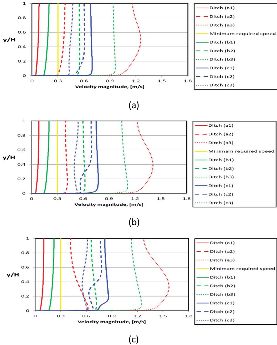
Fig. 15. Vertical flow velocity profile for oxidation ditch bioreactor at nine different locations for the three thrust scenarios: (a) Thrust of 2800 N, (b) Thrust of 3400 N, and (c) Thrust of 4000 N.
