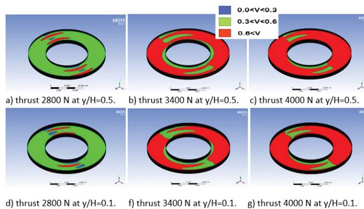
Fig. 16. Velocity contour of the orbital bioreactor in the horizontal section at different height and different impeller thrust forces.
