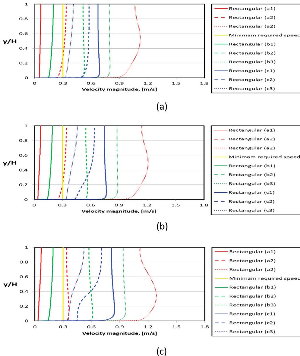
Fig. 12. Vertical flow velocity profile for a rectangular bioreactor at nine different locations for the three thrust scenarios: (a) Thrust of 2800 N, (b) Thrust of 3400 N, and (c) Thrust of 4000 N.
