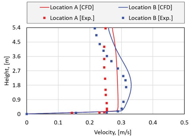
Fig. 8. A comparison between the CFD predictions and the detailed experimental data for the water velocity at two different locations.
