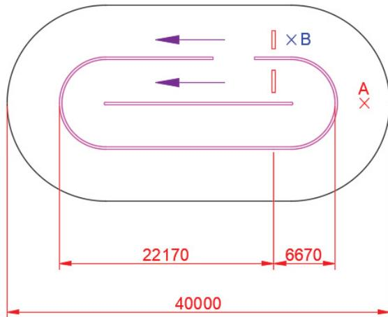
Fig. 7. Illustration of the full-scale ditch and the locations of measurements (dimensions are in mm).
