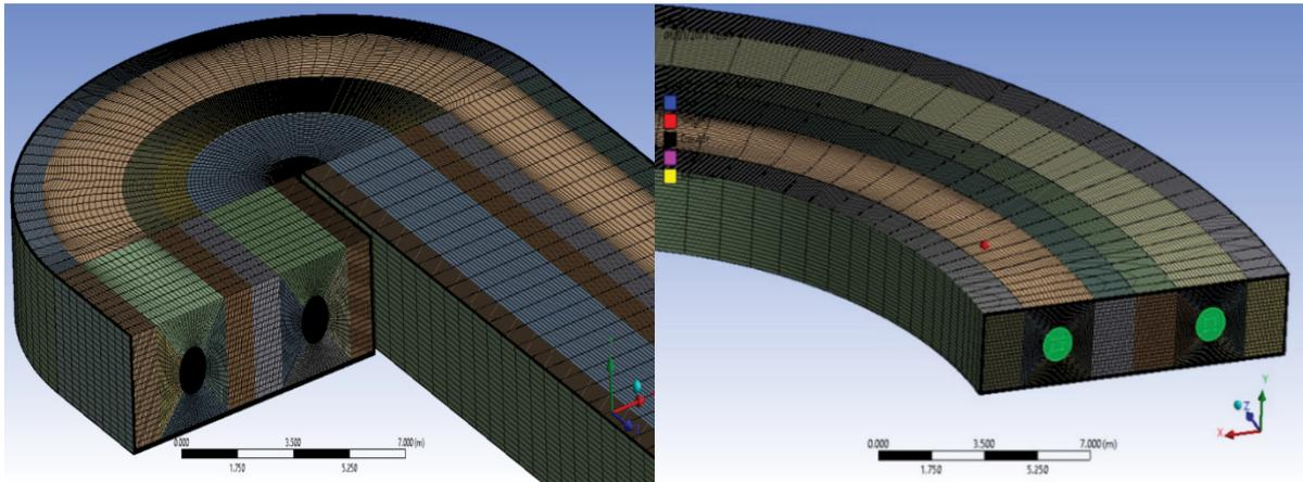
Fig. 4. Grid meshes for bioreactor geometries.
