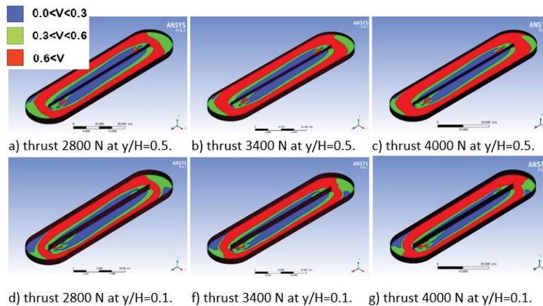
Fig. 13. Velocity contour of the oxidation ditch bioreactor in the horizontal section at different height and different impeller thrust forces.
