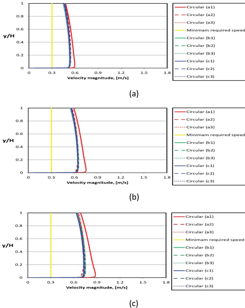
Fig. 18. Vertical flow velocity profile for orbal bioreactor at nine different locations for the three thrust scenarios: (a) Thrust of 2800 N, (b) Thrust of 3400 N, and (c) Thrust of 4000 N.
