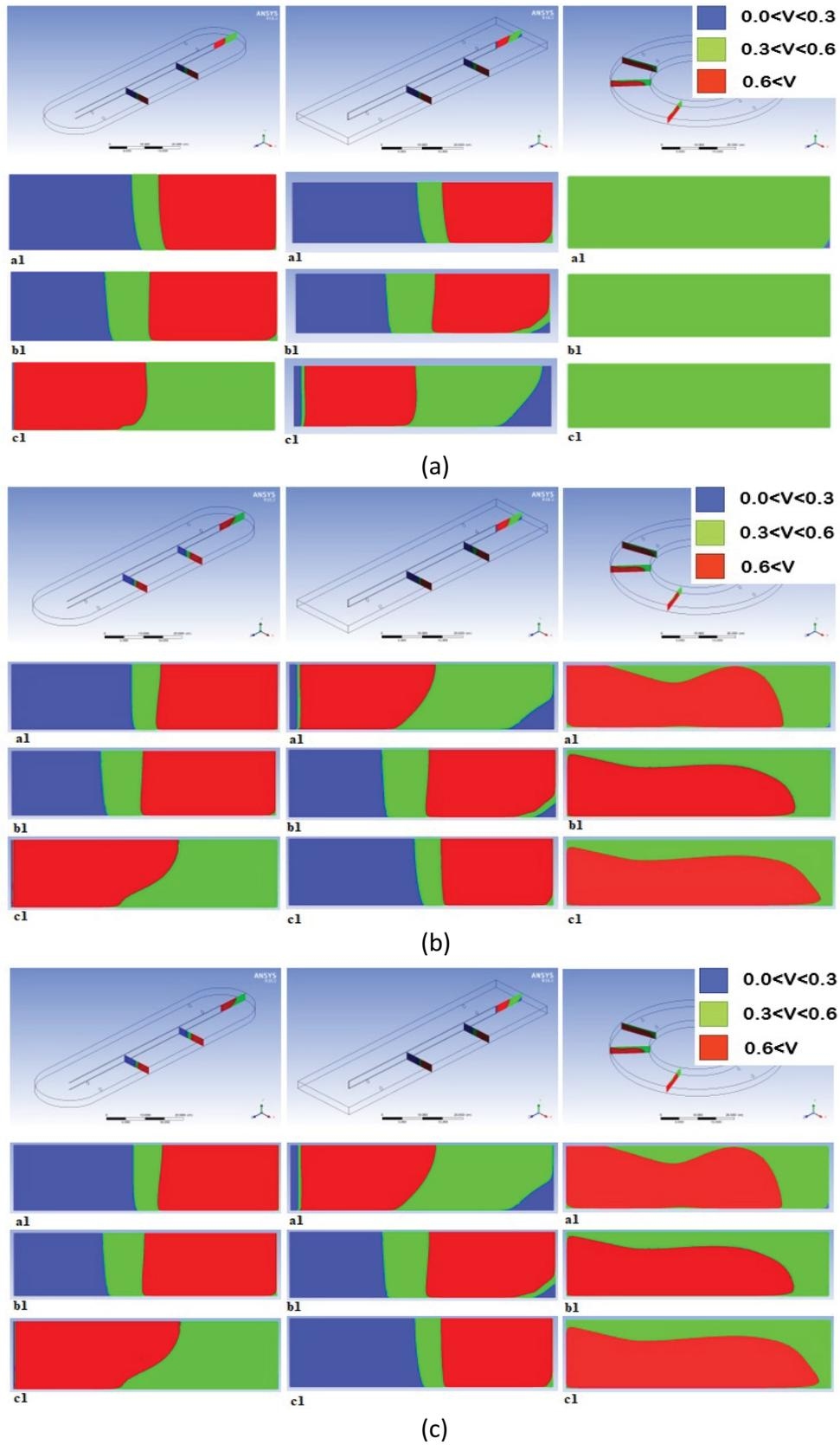
Fig. 19. Flow velocity contour of different bioreactor geometries in the vertical cross section at different impeller thrust forces: (a) Thrust of 2800 N, (b) Thrust of 3400 N, and (c) Thrust of 4000 N.
