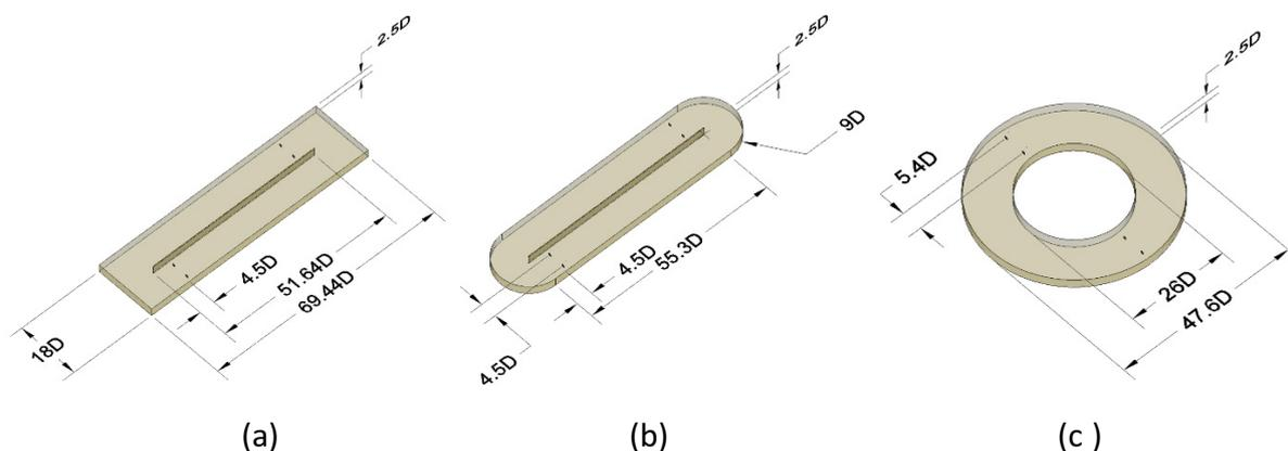
Fig. 3. The features of the three bioreactor geometries: (a) rectangular, (b) oxidation ditch, and (c) orbal.
