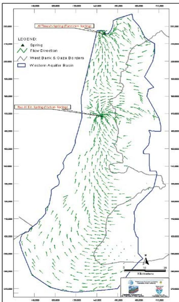
Fig. 5. Directions of groundwater flow of WAB before utilization (putting pumping wells into operation).
