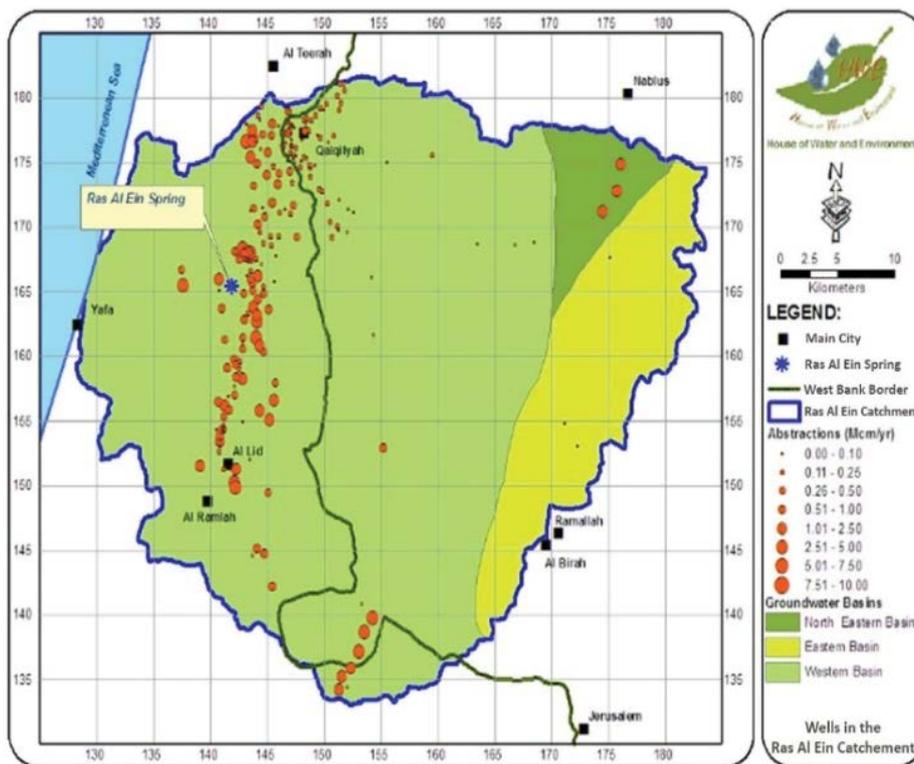
Fig. 3. Location of the main spring (Ras Al-Ain) in the WAB showing heavy pumping around it.
