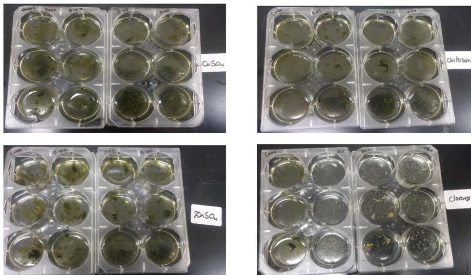
Fig. 8. Lab experiment for algae growth with different chemicals.
