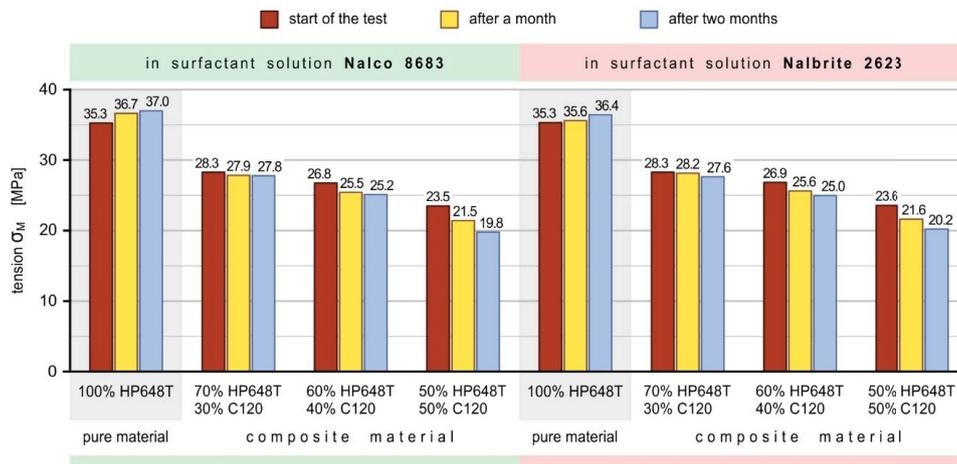
Fig. 4. Comparison of the tensile stress for pure HP648T polypropylene and composites relative to the residence time in NALCO 8683 and NALBRITE 2623 surfactant solutions.
