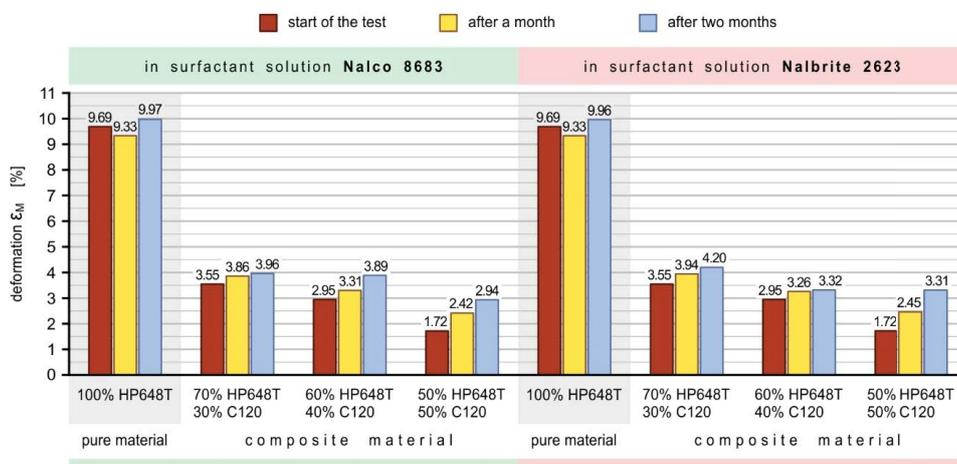
Fig. 5. Comparison of strains during tensile testing for pure HP648T material and HP648T/C120 composites relative to the residence time in NALCO 8683 and NALBRITE 2623 surfactant solutions.
