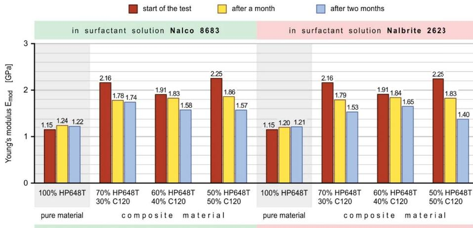
Fig. 3. Comparison of Young's modulus of elasticity during the tensile test – for pure HP648T polypropylene and for composites with different composition relative to the residence time in NALCO 8683 and NALBRITE 2623 surfactant solutions.
