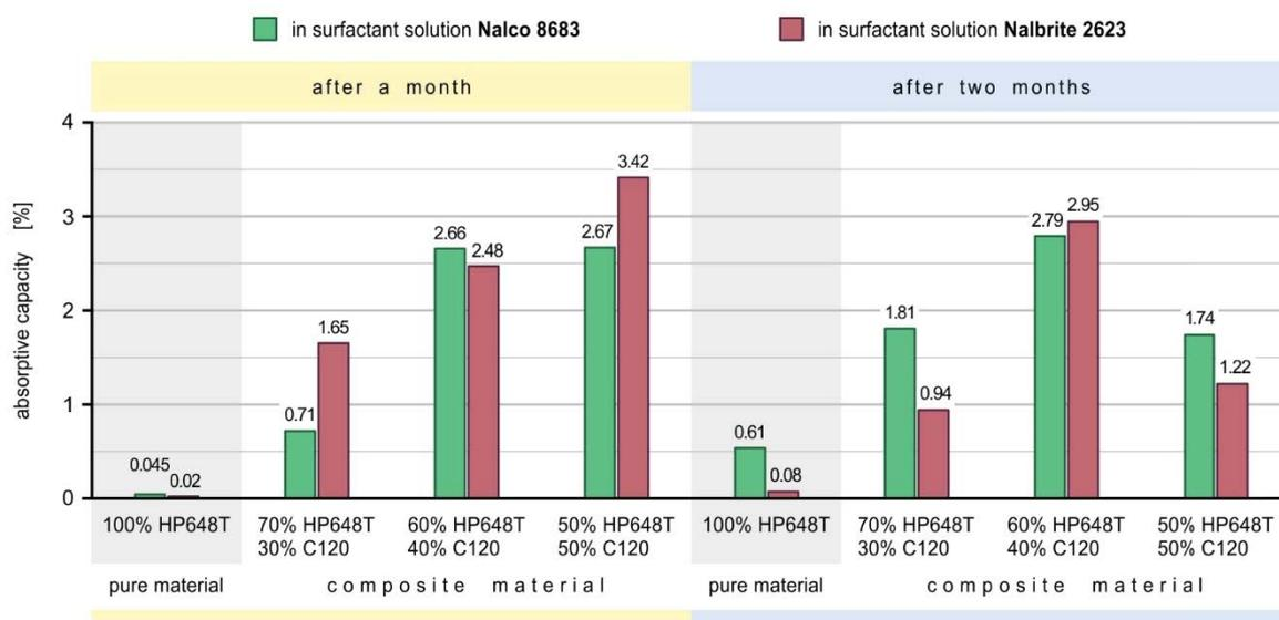
Fig. 1. Summary of absorbency test results after one and two months of exposure to NALCO 8683 and NALBRITE 2623 solutions.
