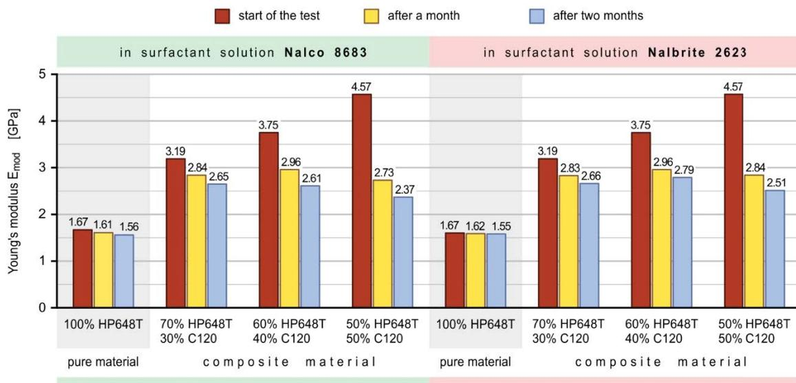
Fig. 2. Comparison of Young’s modulus during the bending test for pure HP648T polypropylene and composites relative to the composition and residence time in NALCO 8683 and NALBRITE 2623 surfactant solutions.
