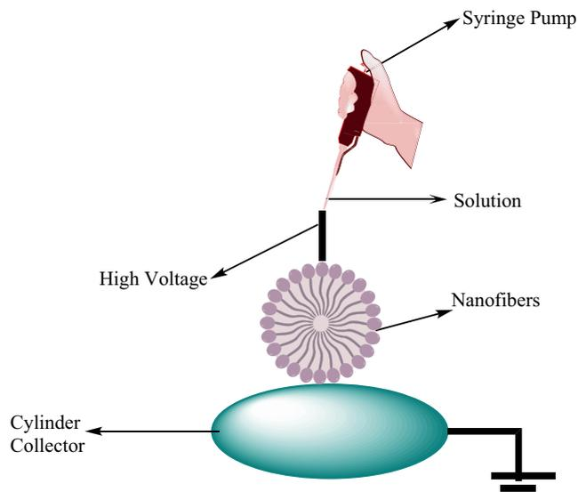
Fig. 3. Electrospinning process [123].
