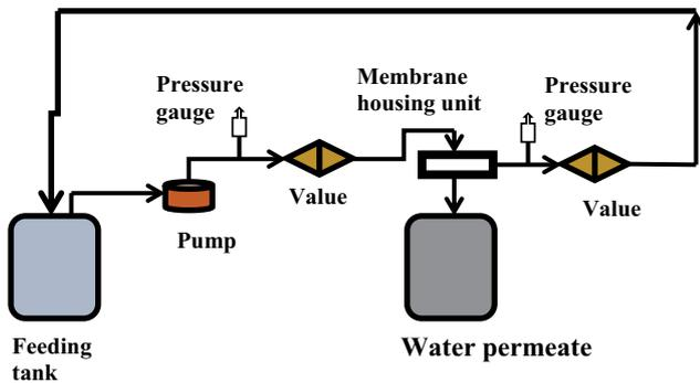
Fig. 1. Laboratory unit for removing salt [60].
