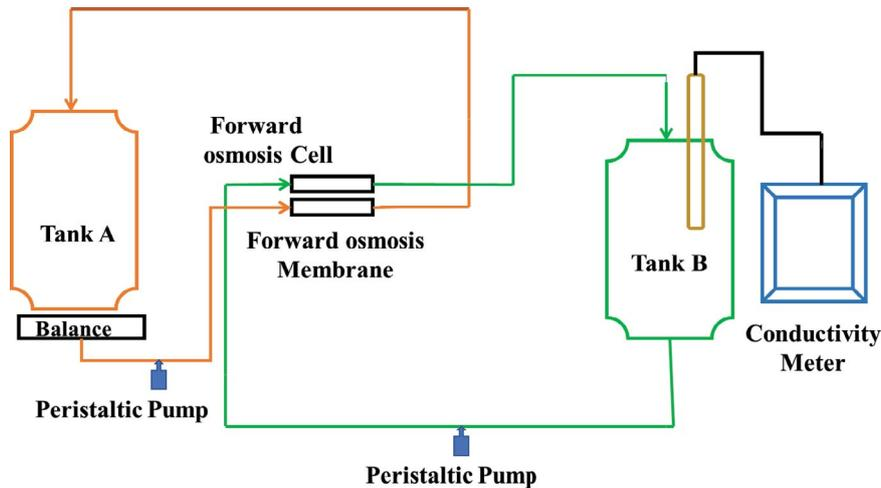
Fig. 2. Flow chart for the forward osmosis process (Tank A = Feed tank, Tank B = Draw tank) [73].
