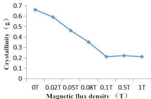
Fig. 3. Average quantity of crystals formed under different magnetic flux densities.
