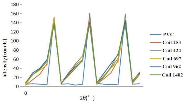
Fig. 4. Diffraction pattern of crystals formed at 0.02 T.
