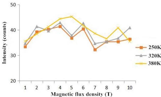
Fig. 13. The relationship between the magnetic flux density and the peak strength at different temperatures (1–10 T).
