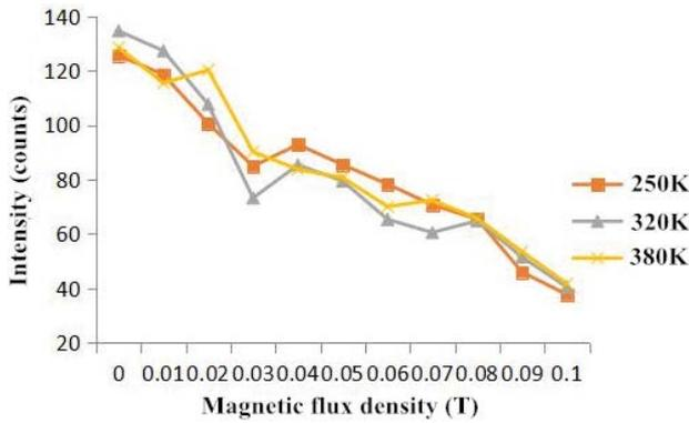
Fig. 11. The relationship between the magnetic flux density and the peak strength at different temperatures (0.01–0.1 T).
