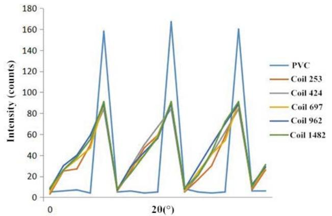
Fig. 7. Diffraction pattern of crystals formed at 0.1 T.
