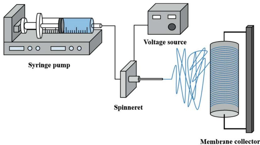
Fig. 4. Schematic diagram for an electrospinning process [71].
