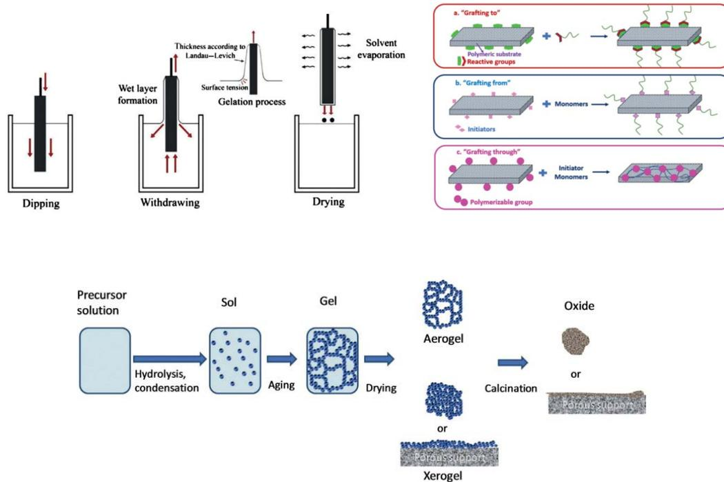
Fig. 3. Schematic drawing for membrane modification techniques (a) dip-coating [Reprinted with permission from Elsevier [63]], (b) surface grafting Suresh et al. [64] and (c) sol-gel method [Reprinted with permission from Elsevier [65]].
