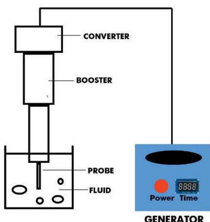
Fig. 2. Schematic of reactor.
