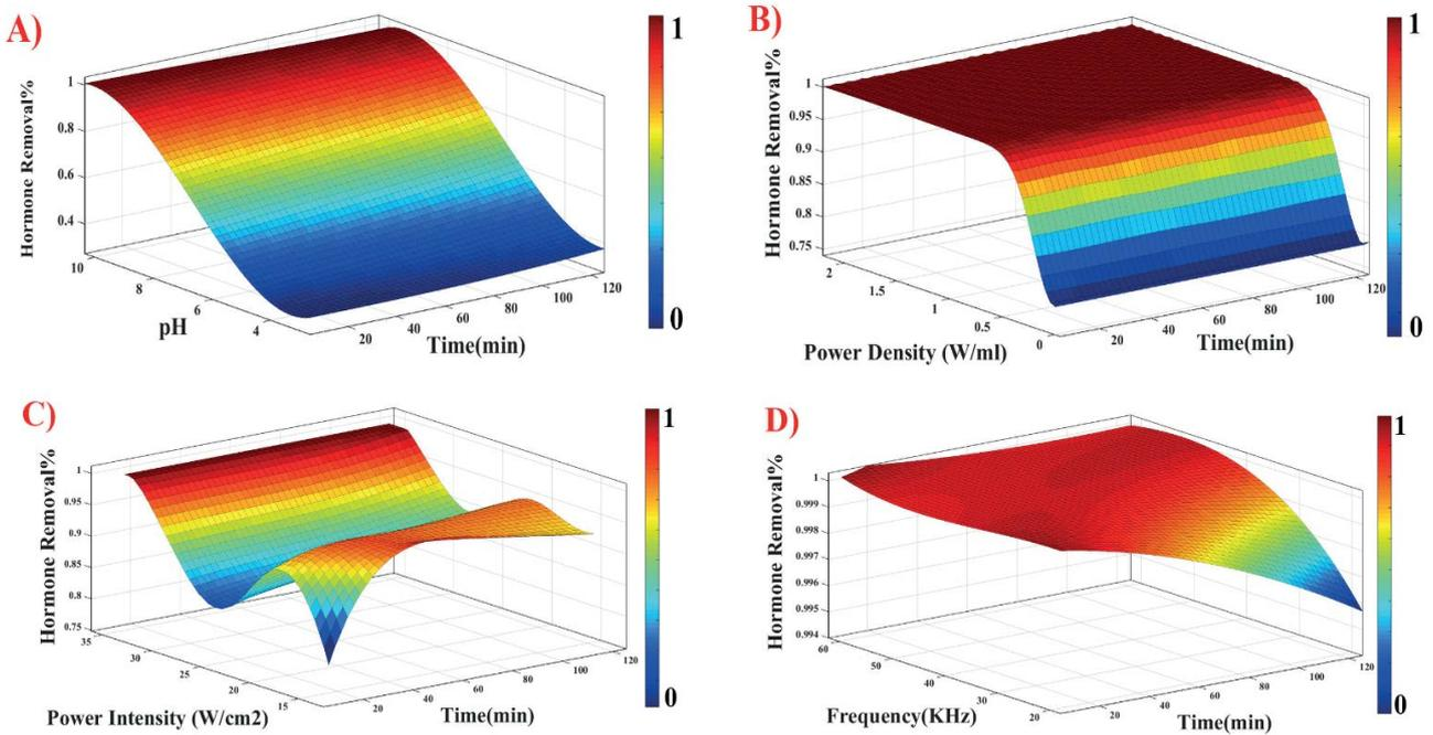
Fig. 6. ANN response surface for (A) pH vs. removal rate of  $E_1$ , (B) power density vs. removal rate of  $E_1$ , (C) power intensity vs. removal rate of  $E_1$ , and (D) frequency vs. removal rate of  $E_1$ .
