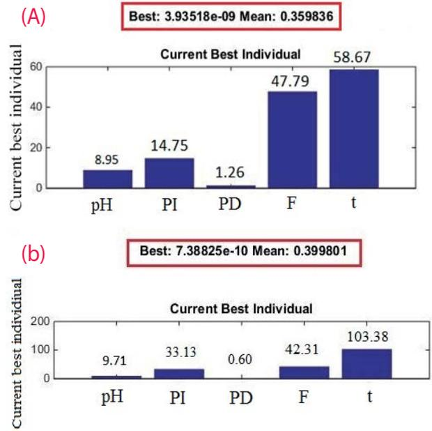
Fig. 5. Genetic algorithm results for: (A) minimum remaining percentage of hormone  $E_1$  and (B) minimum remaining percentage of hormone  $E_2$ .
