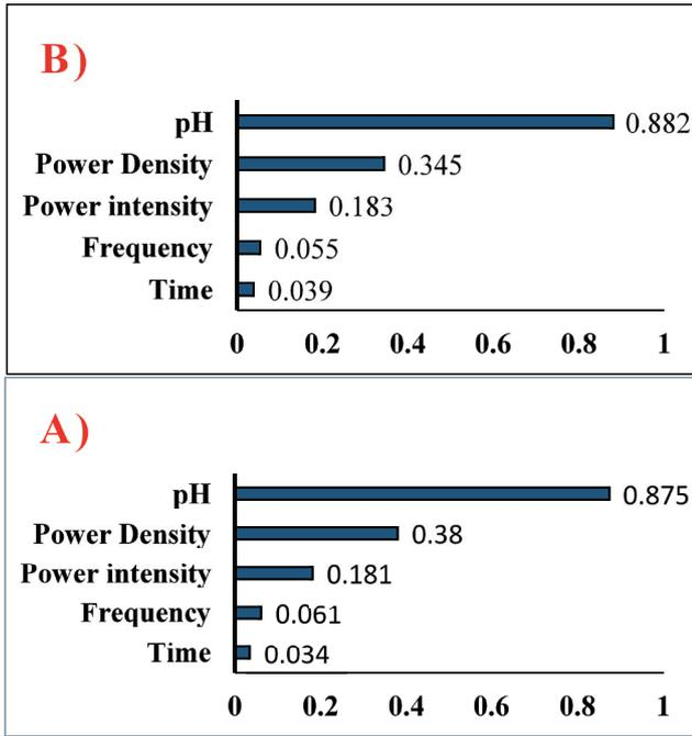
Fig. 4. Tornado graph for sensitivity analysis by standard regression method for (A)  $E_1$  and (B)  $E_2$ .
