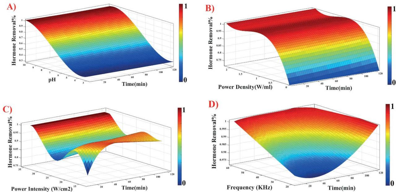
Fig. 7. ANN response surface for (A) pH vs. removal rate of  $E_2$ , (B) power density vs. removal rate of  $E_2$ , (C) power intensity vs. removal rate of  $E_2$ , and (D) frequency vs. removal rate of  $E_2$ .
