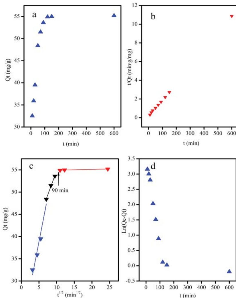
Fig. 7. (a) The biosorption kinetics of *Erwinia* sp. on Pb(II), (b) pseudo-second-order model, (c) Weber–Morris intraparticle diffusion kinetic models and (d) pseudo-first-order model ( $m/V = 1.0$  g/L,  $C_{Pb(II)} = 60$  mg/L,  $T = 303$  K,  $pH = 6.0$ ).
