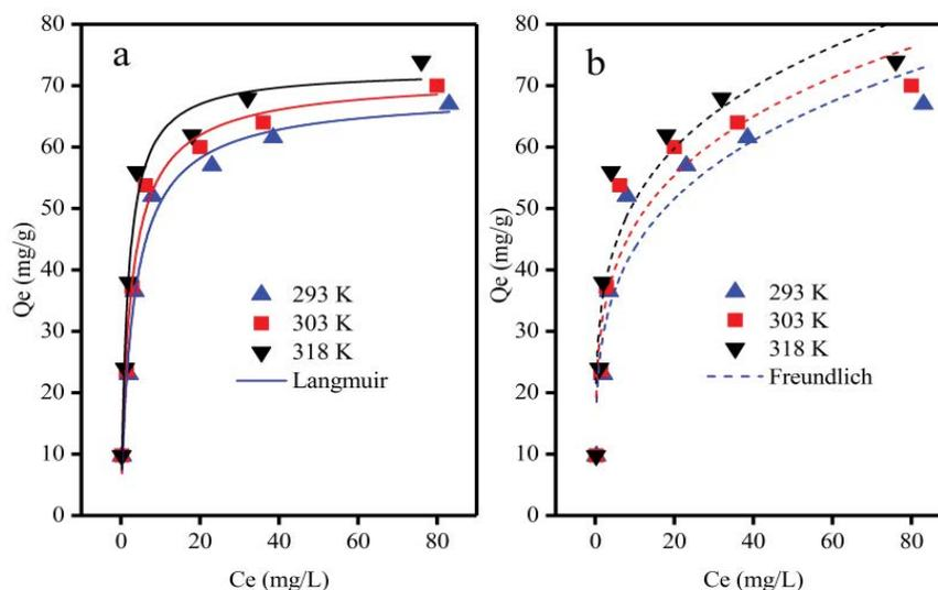
Fig. 6. Biosorption isotherms (a) Langmuir model (b) Freundlich model ( $C_{Pb(II)} = 60$  mg/L, pH = 6.0,  $V = 50$  mL,  $T = 303$  K).
