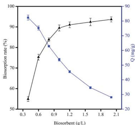
Fig. 5. The effect of biosorbent dosage on biosorption of Pb(II) by *Erwinia* sp. ( $C_{\text{Pb(II)}} = 60$  mg/L, pH = 6.0,  $V = 50$  mL,  $T = 303$  K,  $n = 3$ ).
