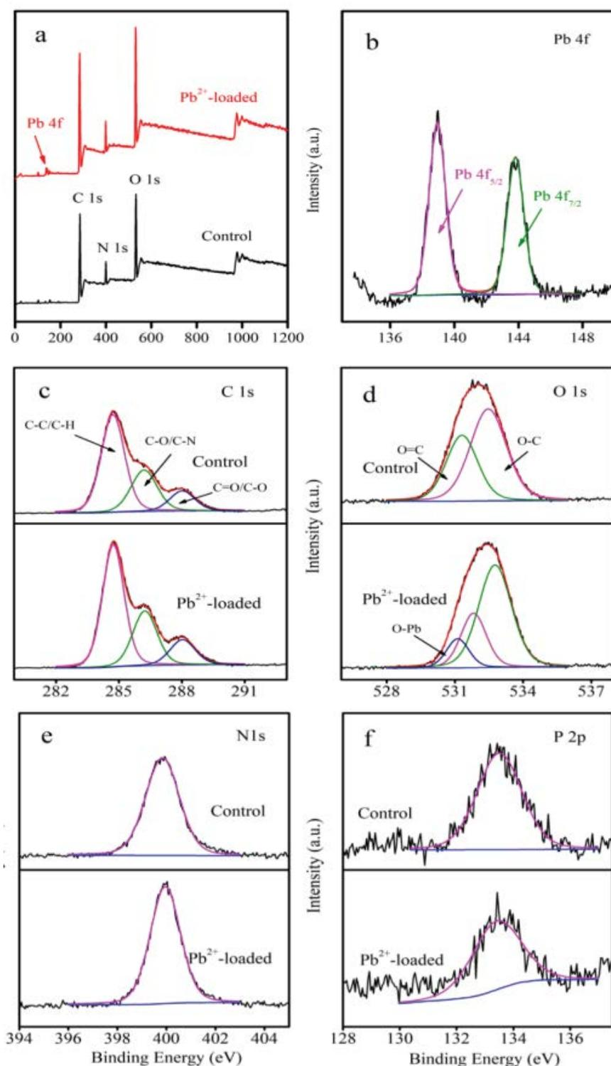
Fig. 3. XPS Intensity curves of Pb biosorption on *Erwinia* sp., (a) total survey scans, (b) Pb4f as a function of the binding energy, (c–d) C 1s, O 1s, N 1s, P 2p.
