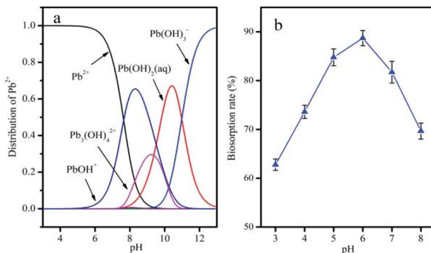
Fig. 4. (a) The relative species distribution of 60 mg/L Pb<sup>2+</sup>; (b) Effect of pH on Pb(II) biosorption by *Erwinia* sp. ( $C_{\text{Pb(II)}} = 60$  mg/L,  $V = 50$  mL,  $m/V = 1.0$  g/L,  $T = 303$  K,  $n = 3$ ).
