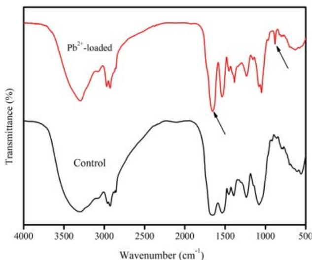
Fig. 2. FT-IR spectra of *Erwinia* sp. before and after biosorption of Pb(II).
