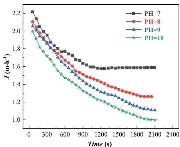
Fig. 7. Curve of the membrane flux under different pH conditions.
