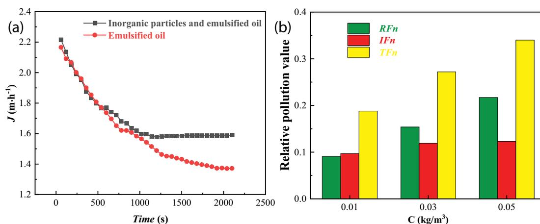
Fig. 10. Fouling of the membrane when emulsified oil and inorganic particles coexist: (a) membrane flux variation curve and (b) fouling of the membrane.
