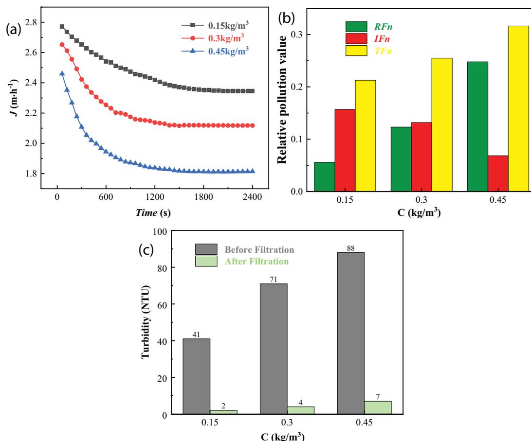
Fig. 3. Effect of different inorganic particle concentrations on the fouling behavior of the membrane: (a) curve of the membrane flux, (b) fouling of the membrane, and (c) change in turbidity before and after filtration.
