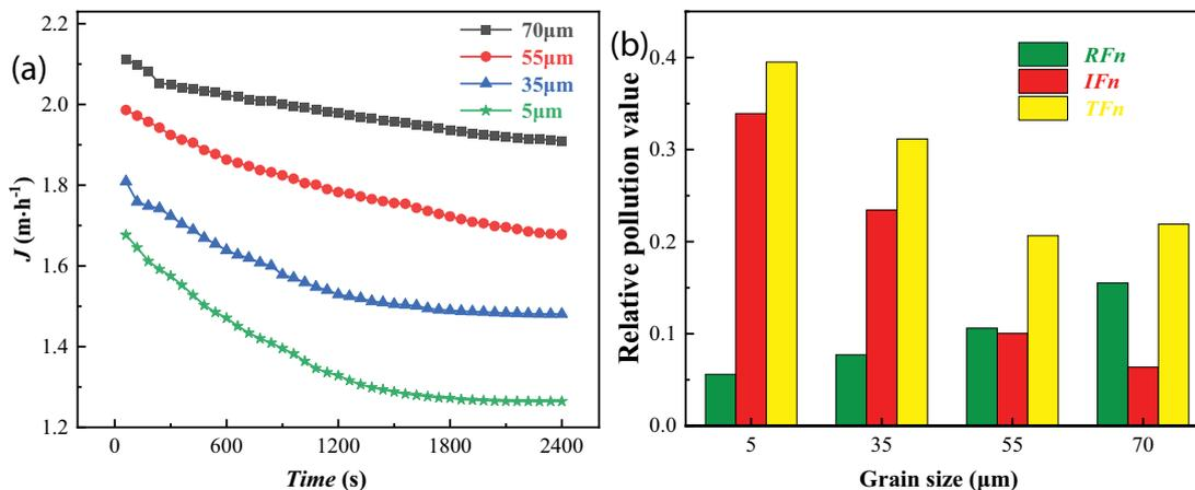
Fig. 5. Effect of different inorganic particle sizes on the fouling behavior of the membrane: (a) curve of the membrane fluxes and (b) fouling of the membrane.
