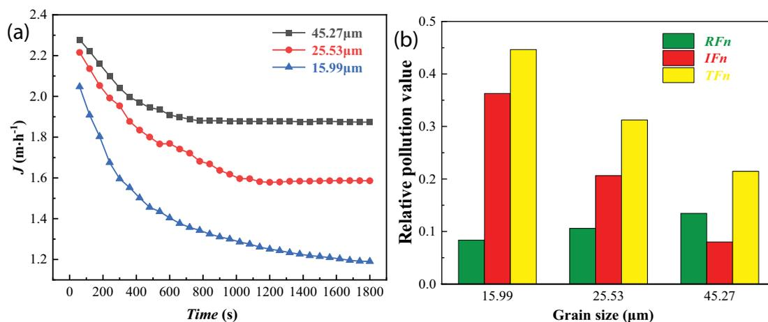
Fig. 8. Effect of different emulsified oil sizes on the fouling behavior of the membrane: (a) curve of the membrane flux and (b) fouling of the membrane.
