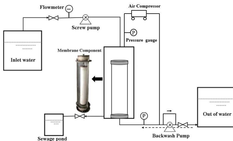
Fig. 1. Schematic diagram of submerged polyethylene porous membrane filtration system.
