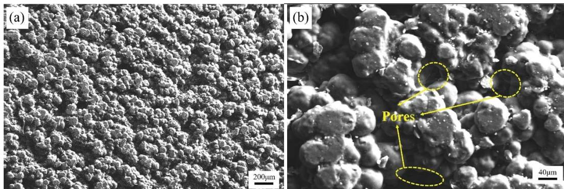
Fig. 2. Micro-SEM images of porous polyethylene tube membrane: (a) outer wall and (b) enlarged view of outer wall.
