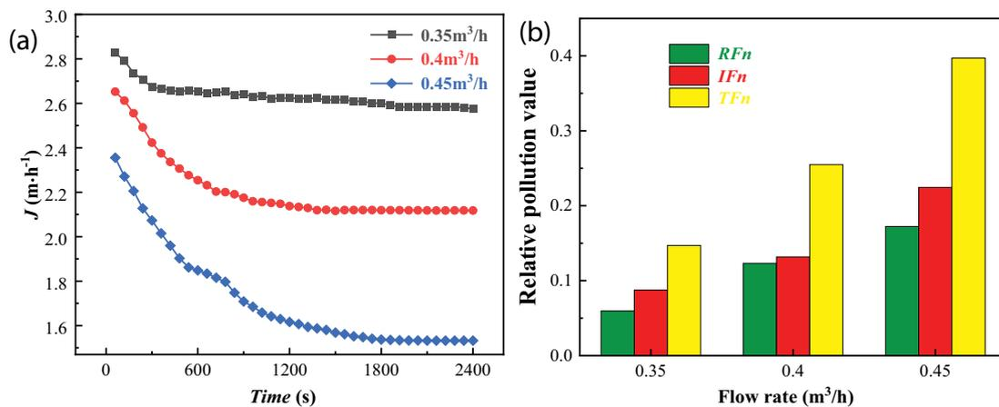
Fig. 4. Effect of different filtration fluxes on the fouling behavior of the membrane: (a) curve of the membrane fluxes and (b) fouling of the membrane.
