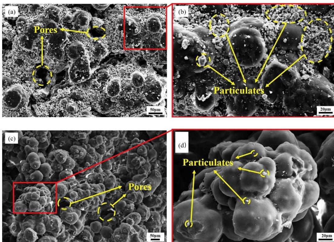
Fig. 9. Micro-SEM images of the contaminated polyethylene tube membrane (a) outer wall, (b) enlargement of figure (a), (c) inner wall, and (d) enlargement of figure (c).
