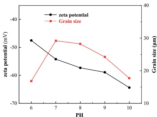
Fig. 6. Effect of pH on zeta potential and particle size of emulsified oil.
