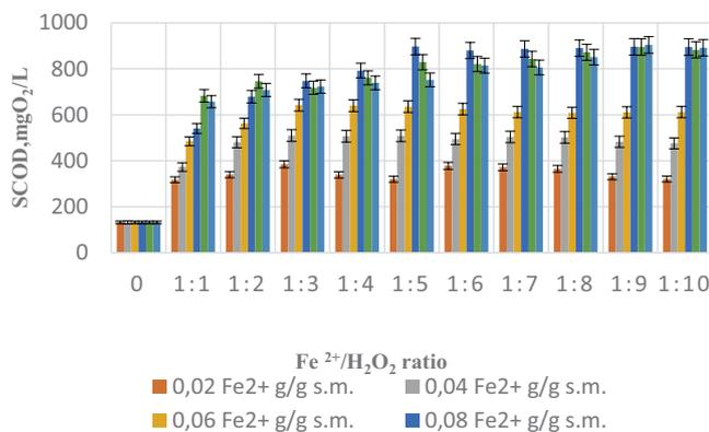
Fig. 1. Effect of Fenton's reagent on SCOD values depending on the ratio of chemical reagents used.
