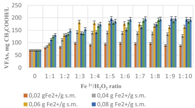
Fig. 2. Effect of Fenton's reagent on VFA concentration depending on the ratio of chemical reagents.
