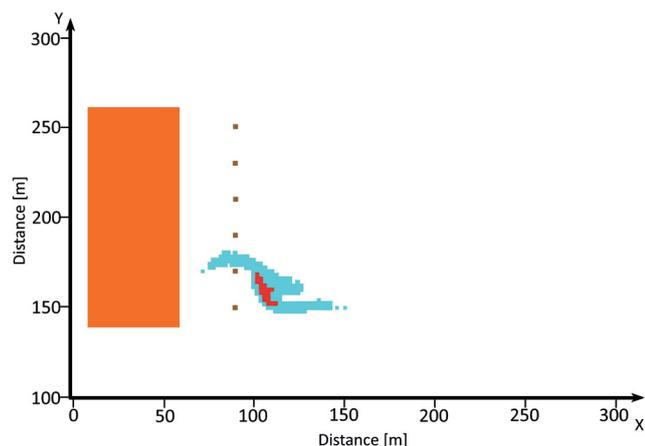
Fig. 10. System of six wells monitoring contamination from a landfill in a heterogeneous aquifer.
