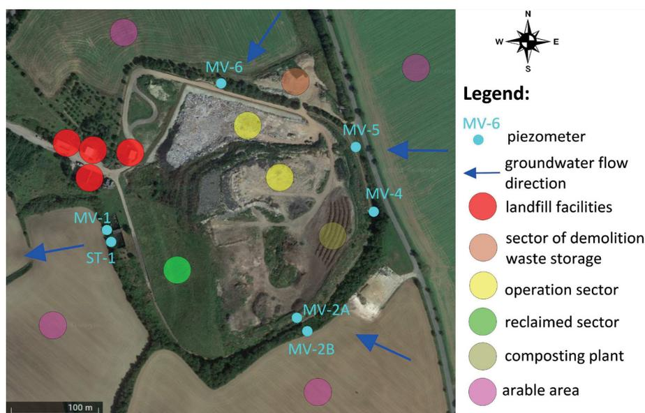
Fig. 2. Monitoring network of the groundwater quality at the Zdounky landfill, together with a view of the landfill's waste compartments.
