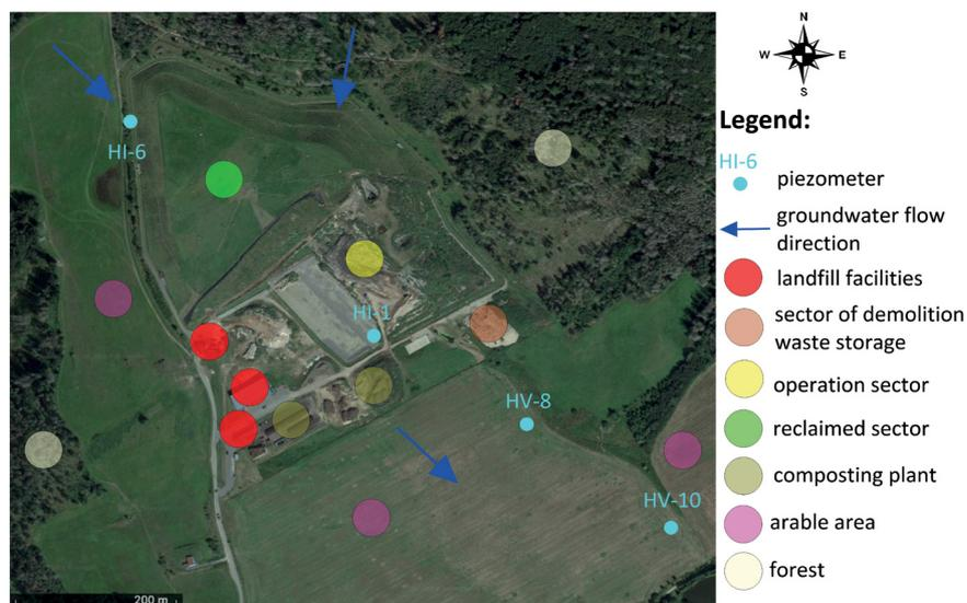
Fig. 3. Monitoring network of the groundwater quality at the Petřůvky landfill together with a view of the landfill's waste compartments.
