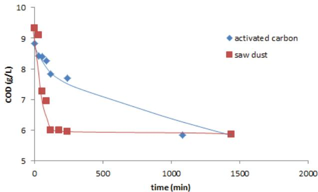
Fig. 3. Adsorption kinetics for both activated carbon and sawdust particles mixed with dairy wastewater (dose 5 g/100 mL) at a stirring rate of 70 rpm.
