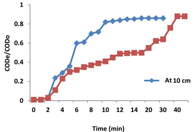
Fig. 4. Breakthrough curves of the adsorption treatment of dairy wastewater in packed bed of sawdust at two different bed heights (10 and 30 cm).
