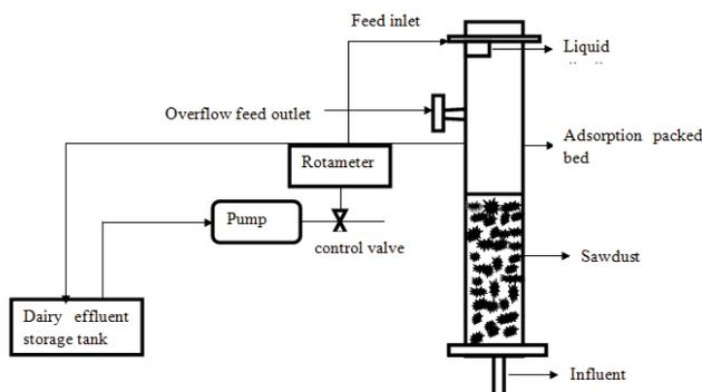
Fig. 2. Schematic representation of the continuous adsorption packed-bed setup.
