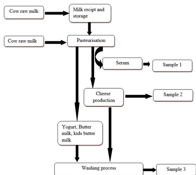
Fig. 1. Process flow chart for dairy industry showing the locations from which the wastewater samples were collected.
