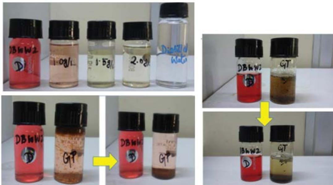
Fig. 10. Dyebath (DBWW2) wastewater decolorization using green iron particles.
