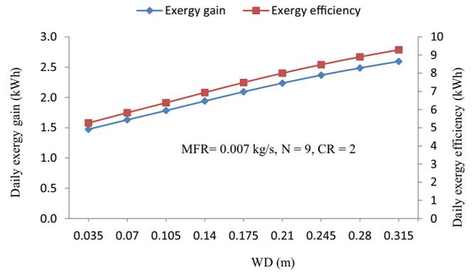
Fig. 17. Dissimilarity of daily exergy gain and daily exergy efficiency with WD at selected values of N, CR and MFR for NCPCEC-DS.
