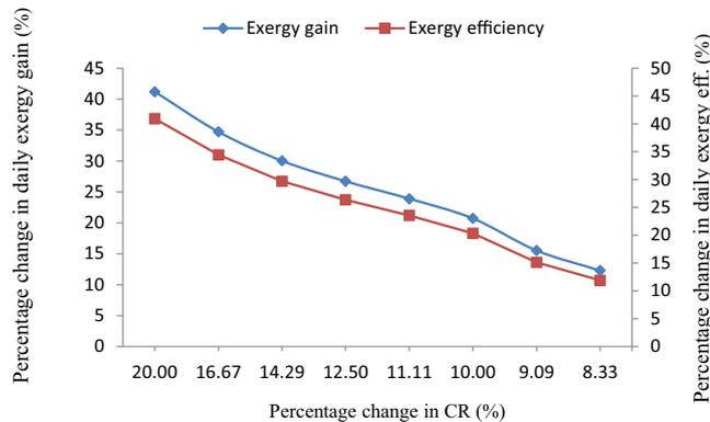
Fig. 20. Sensitivity of daily exergy gain and exergy efficiency with regard to CR at selected values of N, WD and MFR for NCPCEC-DS.
