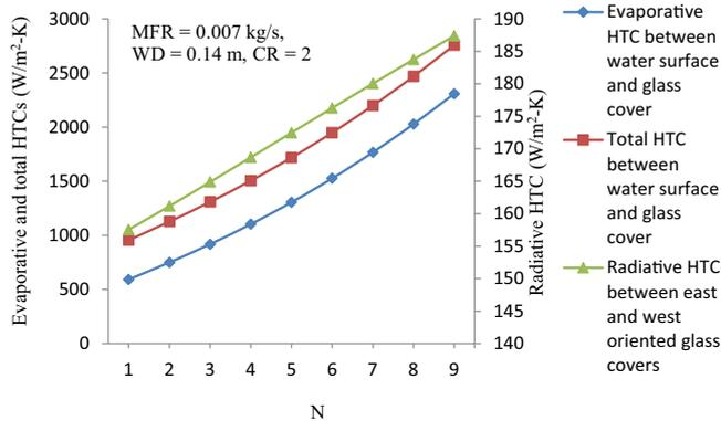
Fig. 7. Dissimilarity of daily heat transfer coefficients (HTCs) with N at selected values of MFR, CR and WD for NCPCEC-DS.
