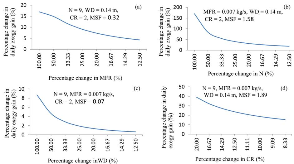
Fig. 12. Sensitivity of daily exergy gain with regard to (a) MFR, (b) N, (c) WD and (d) CR for collector maintaining other parameters at the input of system constant.
