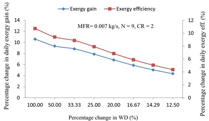
Fig. 18. Sensitivity of daily exergy gain and exergy efficiency with regard to WD at selected values of N, CR and MFR for NCPCEC-DS.
