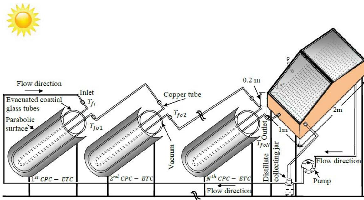
Fig. 1.  $N$  identical CPCETCs integrated double slope solar distiller unit (NCPCETC-DS).
