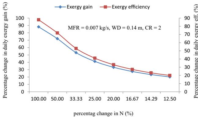
Fig. 16. Sensitivity of daily exergy gain and exergy efficiency with regard to N at selected values of N, CR and MFR for NCPCEC-DS.
