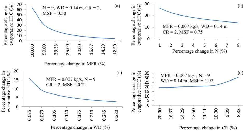
Fig. 10. Sensitivity of daily HTC with regard to (a) MFR, (b) N, (c) WD and (d) CR for NCPETC-DS maintaining other parameters at the input of system constant.
