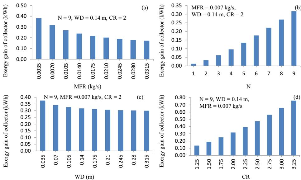
Fig. 11. Dissimilarity of daily exergy gain with (a) MFR, (b) N, (c) WD and (d) CR for collector maintaining other parameters at the input of system constant.
