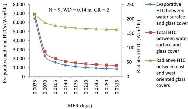
Fig. 6. Dissimilarity of daily heat transfer coefficients (HTCs) with MFR at selected values of N, CR and WD for NCPCEC-DS.
