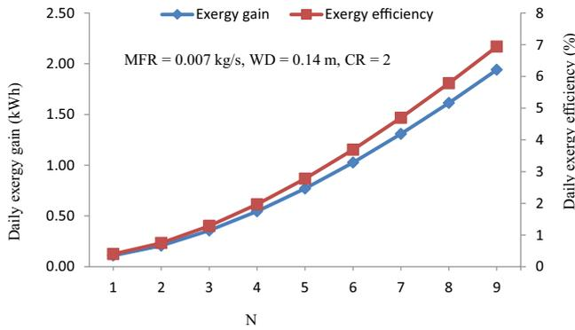
Fig. 15. Dissimilarity of daily exergy gain and daily exergy efficiency with N at selected values of MFR, CR and WD for NCPCEC-DS.
