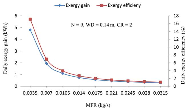
Fig. 13. Dissimilarity of daily exergy gain and daily exergy efficiency with MFR at selected values of N, CR and WD for NCPCEC-DS.
