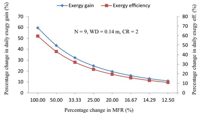
Fig. 14. Sensitivity of daily exergy output and daily exergy efficiency with regard to MFR at selected values of N, CR and WD for NCPCEC-DS.
