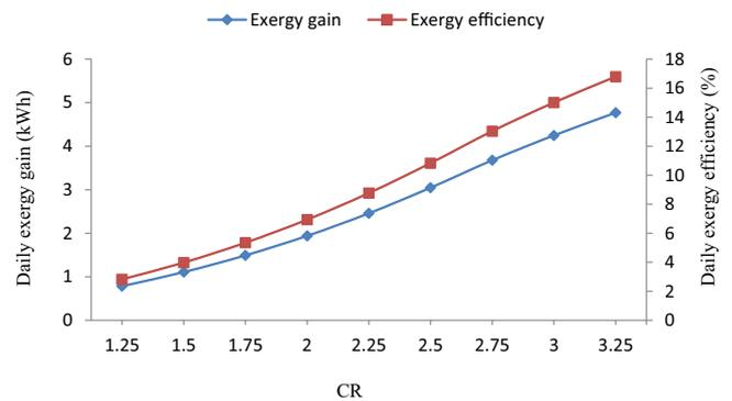
Fig. 19. Dissimilarity of daily exergy gain and exergy efficiency with CR at selected values of N, WD and MFR for NCPCEC-DS.
