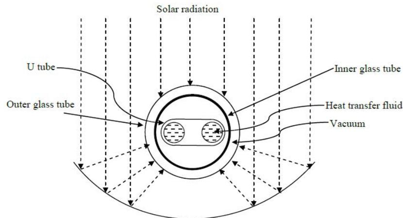
Fig. 2. Cross-section side view of the first CPCETC.
