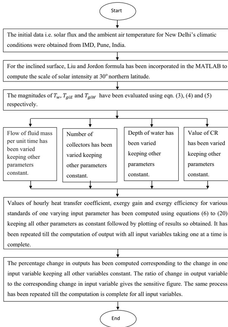
Fig. 4. Flow chart of methodology for carrying out sensitivity analysis for NCPCEC-DS.
