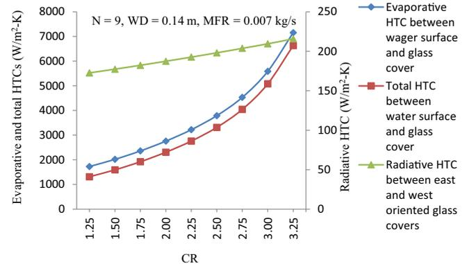
Fig. 9. Dissimilarity of daily heat transfer coefficients (HTCs) with CR at selected values of N, CR and MFR for NCPCEC-DS.
