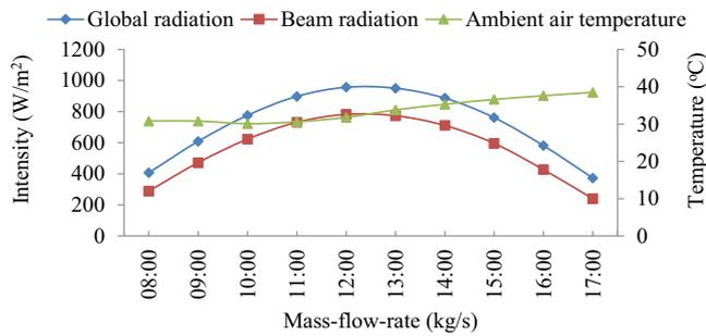
Fig. 5. Hourly variation of intensity and ambient air temperature for a typical day in the month of May.
