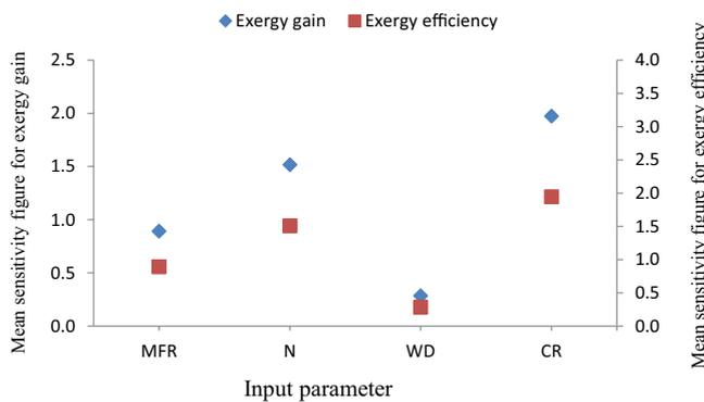
Fig. 21. Comparative sensitivity figure of exergy gain as well as exergy efficiency with respect to input parameter (MFR/N/WD/CR) for NCPCEC-DS.
