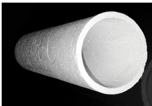
Fig. 2. Thin-walled tube specimen made of PCC.
