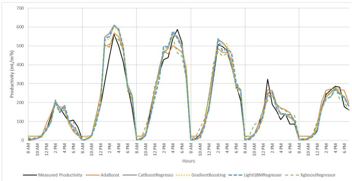
Fig. 7. Comparison between measured and predicted solar still productivity by five boosting models based on the testing datasets.
