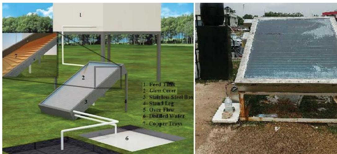
Fig. 1. Inclined system with the main components.
