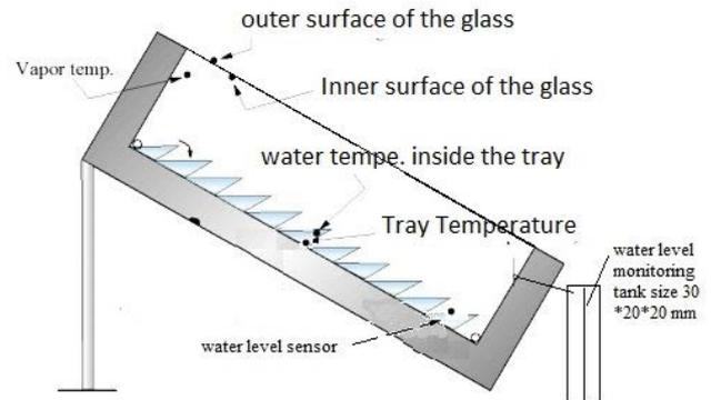
Fig. 2. Position of different points for measuring temperature variations.
