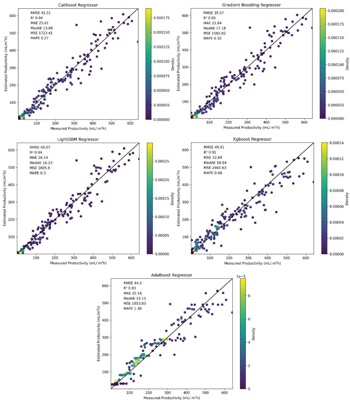
Fig. 8. Scatter plots show the differences between the measured and estimated productivity for the five models: CatBoost, AdaBoost, XGBoost, gradient boosting, and LightGBM.
