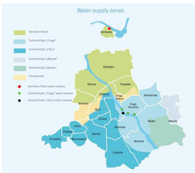
Fig. 1. Water supply zones with marked water intakes [26].
