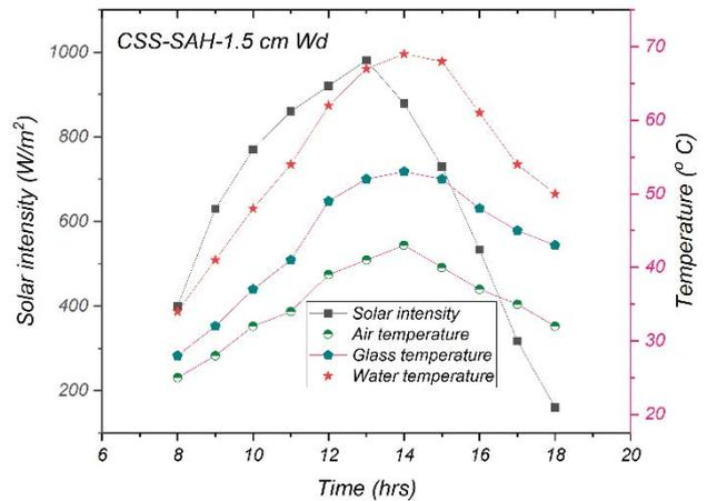
Fig. 9. Hourly plots of CSS-SAH at 1.5 cm  $W_d$  temperature profile and input parameters.
