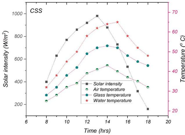
Fig. 6. Hourly plots of CSS temperature profile and input parameters.
