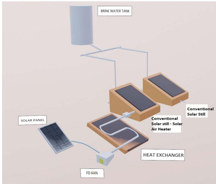
Fig. 3. Schematic of the CSS with heat exchanger and SAH.
