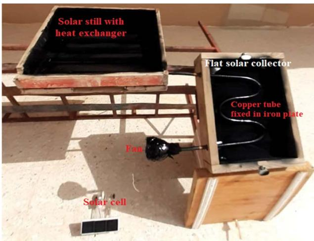
Fig. 4. Photo of the CSS with heat exchanger and SAH.
