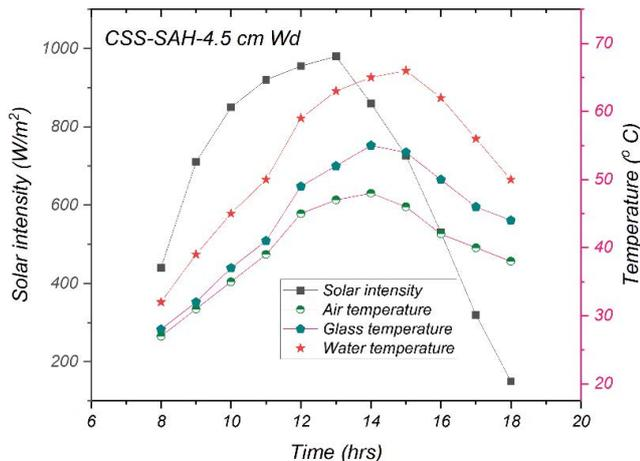
Fig. 11. Hourly plots of CSS-SAH at 4.5 cm  $W_d$  temperature profile and input parameters.
