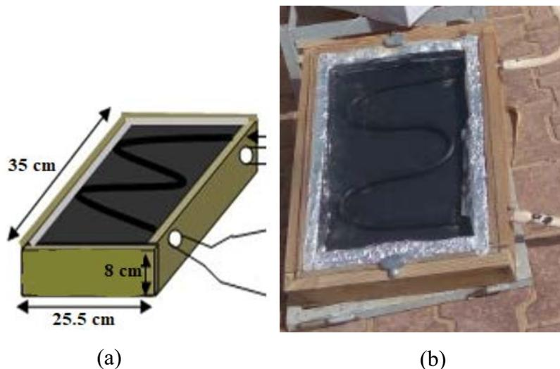
Fig. 2. Flat solar collector (a) Schematic presentation of SAH and (b) Photo of the SAH.
