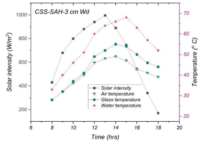
Fig. 10. Hourly plots of CSS-SAH at 3 cm  $W_d$  temperature profile and input parameters.
