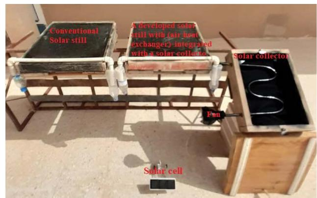
Fig. 5. Photograph of the CSS, CSS with heat exchanger, and SAH.
