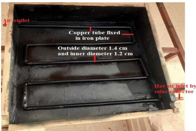
Fig. 1. Solar still with the heat exchanger of the studied system.
