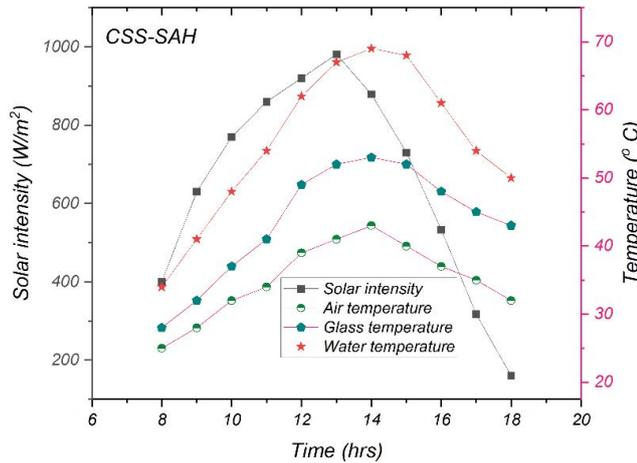
Fig. 7. Hourly plots of CSS-SAH temperature profile and input parameters.
