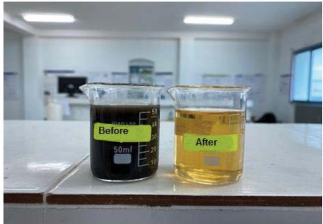
Fig. 18. Real textile effluents before and after electrocoagulation treatment.
