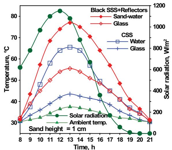
Fig. 7. Solar irradiation and temperatures profiles for BSSS with mirrors.
