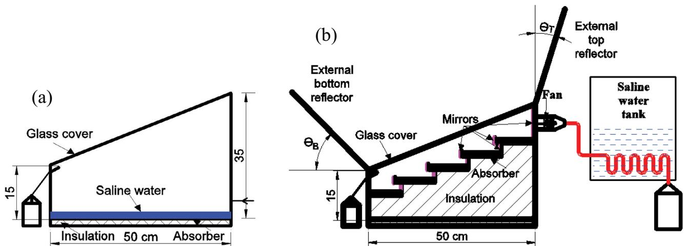
Fig. 2. Schematic drawing of setup. (a) Conventional solar still and (b) black sand stepped solar still with reflectors and fan.
