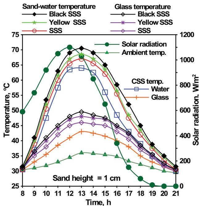
Fig. 3. Temperatures and solar irradiation for solar stills at sand height 1 cm.
