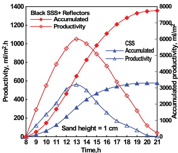
Fig. 8. Total and hourly yields for tested stills at sand height 1 cm with mirrors.
