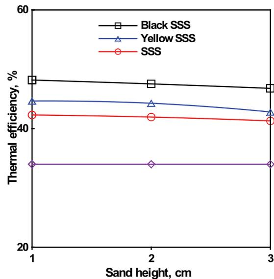
Fig. 6. Efficiency of stills at different sand bed height.
