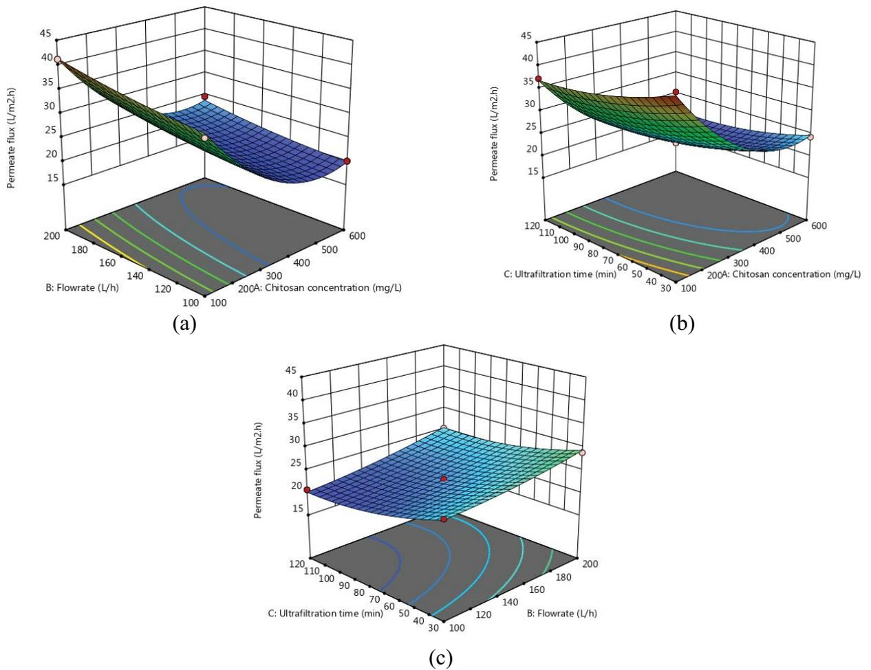
Fig. 2. Variation of permeate flux with (a) flow rate and chitosan concentration at 75 min ultrafiltration time, (b) ultrafiltration time and chitosan concentration at 150 L/h flowrate and (c) ultrafiltration time and flowrate, and at 350 mg/L chitosan concentration.
