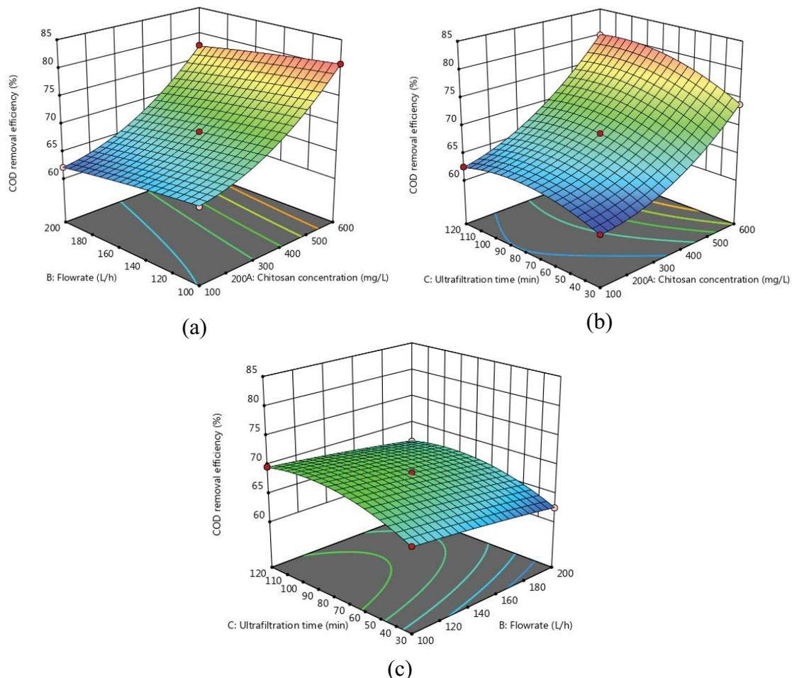
Fig. 3. Variation of chemical oxygen demand removal with (a) flow rate and chitosan concentration at 75 min ultrafiltration time, (b) ultrafiltration time and chitosan concentration at 150 L/h flowrate and (c) ultrafiltration time and flowrate with 350 mg/L chitosan concentration.
