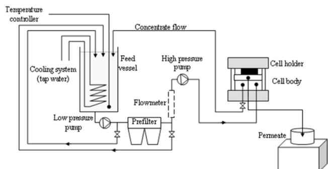
Fig. 1. Schematic flow diagram of the experimental set-up.
